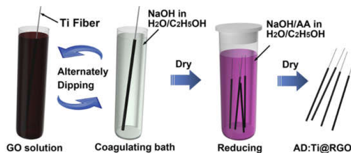
Figure 14. Schematic representation of the synthesis of AD:Ti@RGO via the drying and dipping method for applications in supercapacitors. Reproduced with permission from [210]. IScience, 2020.
