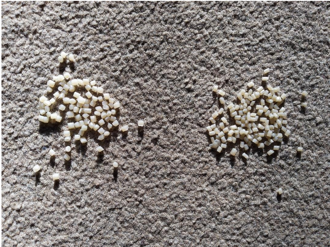
Fig. 15: Two low-density polythene (LDPE) pellet samples are presented. The one on the left – of lighter and 'cleaner' tone – is graded as 'high' quality, the sample on the right – slightly darker and with more particulate admixture – is 'medium' quality. They are priced at Rs.75/kg and Rs.65/kg respectively as of January 2021. The recyclers can 'see and tell' their differences. On rare occasions, they would bite a pellet and know its quality and price. Courtesy: Author
