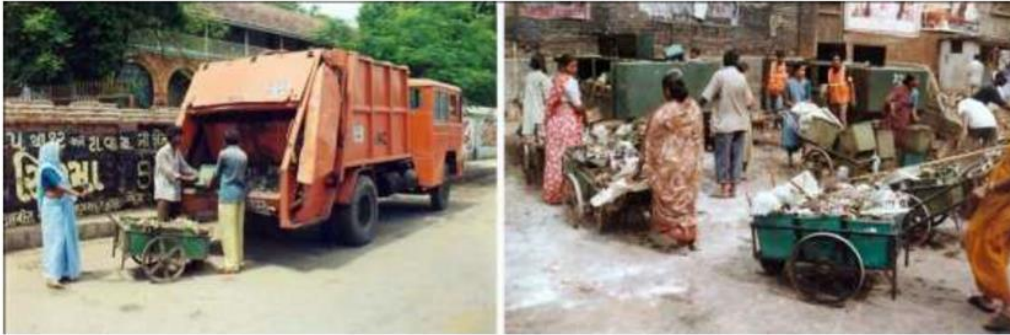
Transfer of MSW from Street Sweeping into Compactor & Secondary Collection Bin
