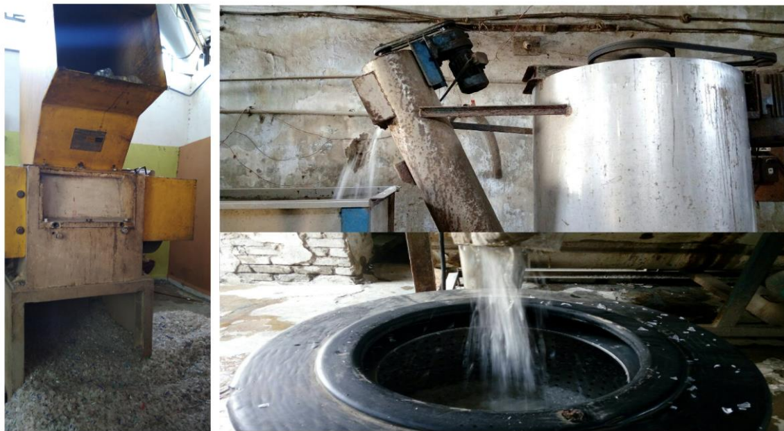
Fig. 35: PET 'flakes' produced at the collective's 'integrated' SWM site (left) are transported in tightly-tied raffia sacks to commercial 'recyclers' (right) for cleaning and drying (via alkaline baths and centrifugal rotation in the picture). The two images on the right are from one such partner situated at a small warehouse remodelled from the ruins of an old textile mill in Naroda, whose specialisation lay exclusively in PET processing. Courtesy: Author
