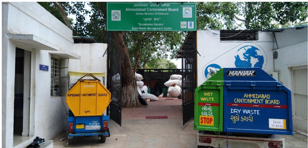
Fig. 27: On the right is a typical door-to-door waste collection vehicle, colour-coded with separate dry-wet waste compartments. Courtesy: Author
