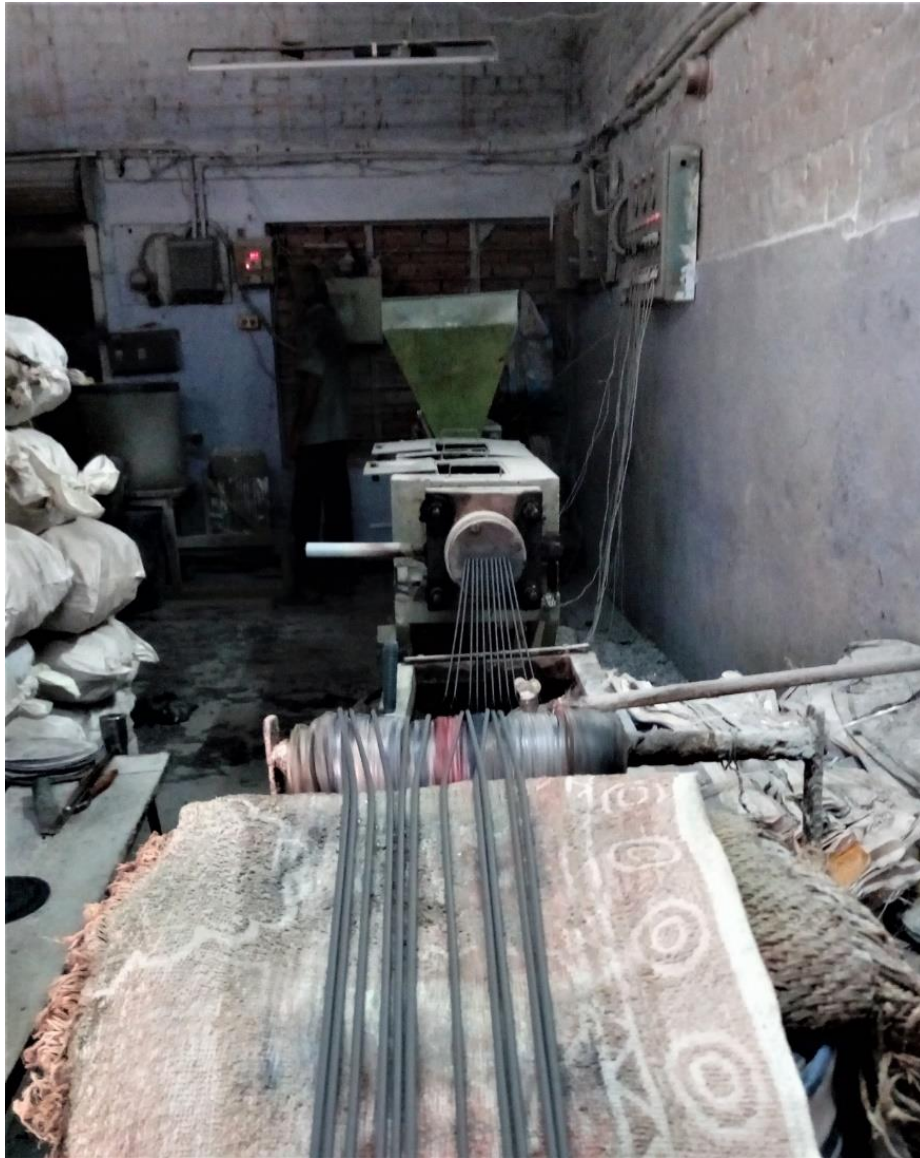
Fig. 14: A polythene pellet-making unit in Rakhiyal with daily capacity of about 500 kg. Melted polythene ‘threads’ are extruded through sieves (of variable diameter) passed under cold water to solidify before these solidified threads are chopped off by a time-calibrated mechanical axe to prepare pellets. Courtesy: Author
