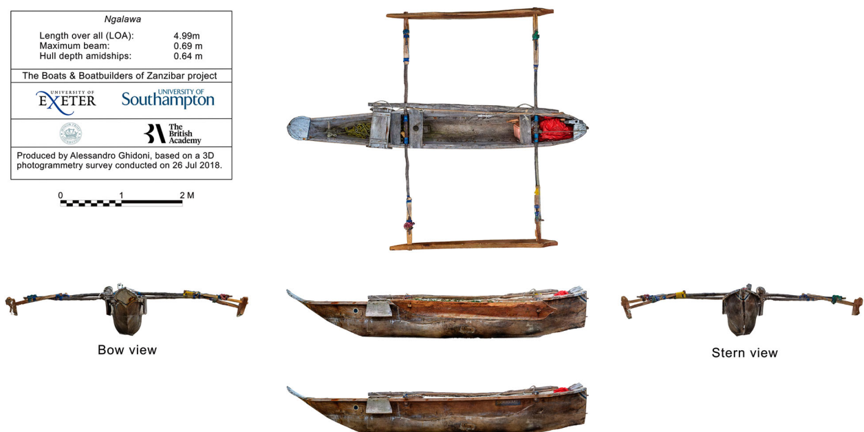
Figure 2. Orthographic views of a ngalawa recorded at Marahubi, Unguja, in July 2018, based on a 3D photogrammetry survey (Image: Alessandro Ghidoni).
