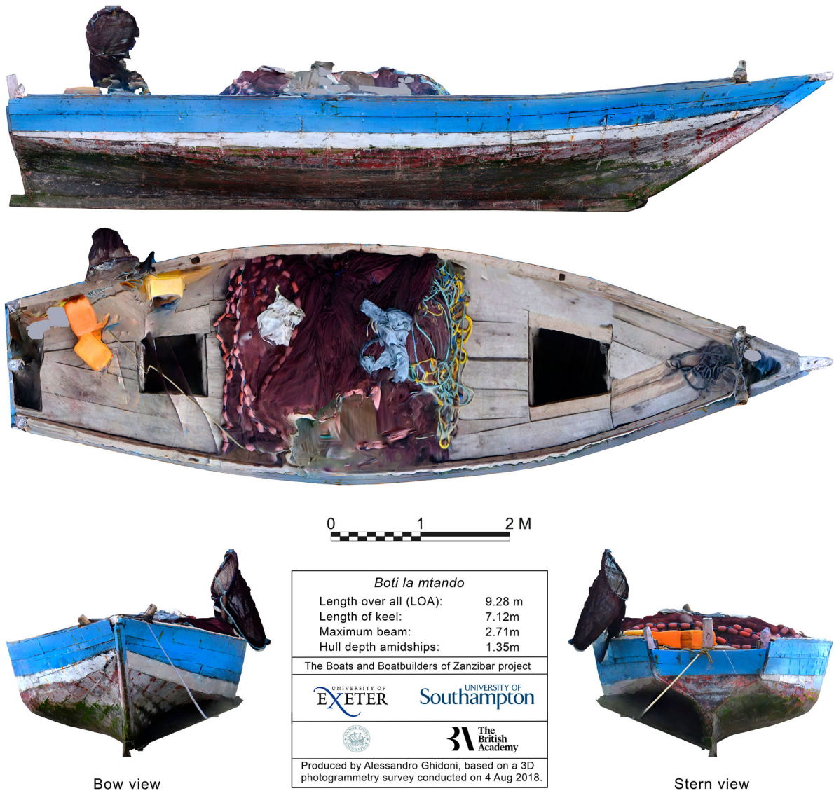
Figure 19. Orthographic views of a plank-built boti la mtando fishing boat, recorded at Marahubi, Unguja, in August 2018, based on a 3D photogrammetry survey (Image: Alessandro Ghidoni).
