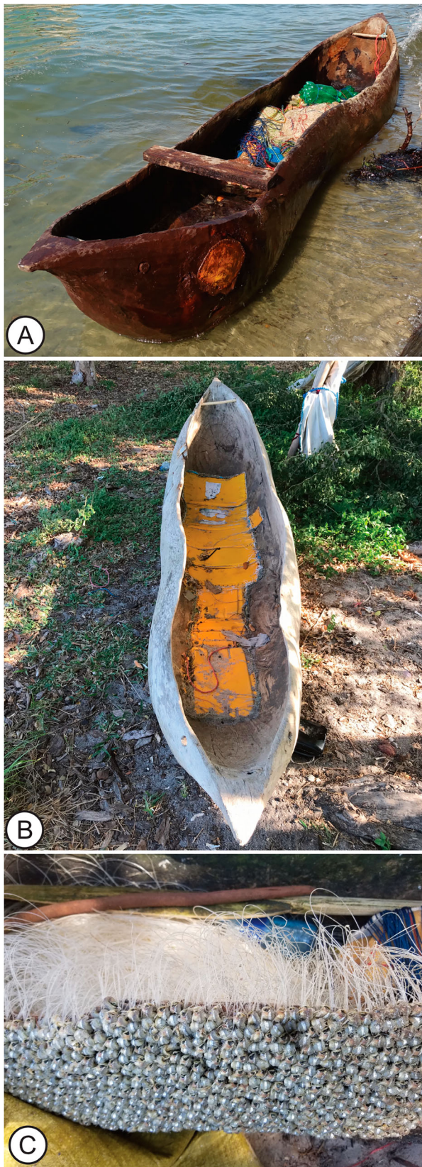
Figure 8. Lake Nyasa mtumbwis ( vuwatu ) (A) on the shore at Milingotini; (B) at Milingotini showing extensive use of yellow-polythene repair patchwork; (C) long-line fishhooks arrayed on the gunwale of a boat at Bagamoyo, February 2020 (Images: John P. Cooper; Lucy Blue; Sinyati R. Mark).
