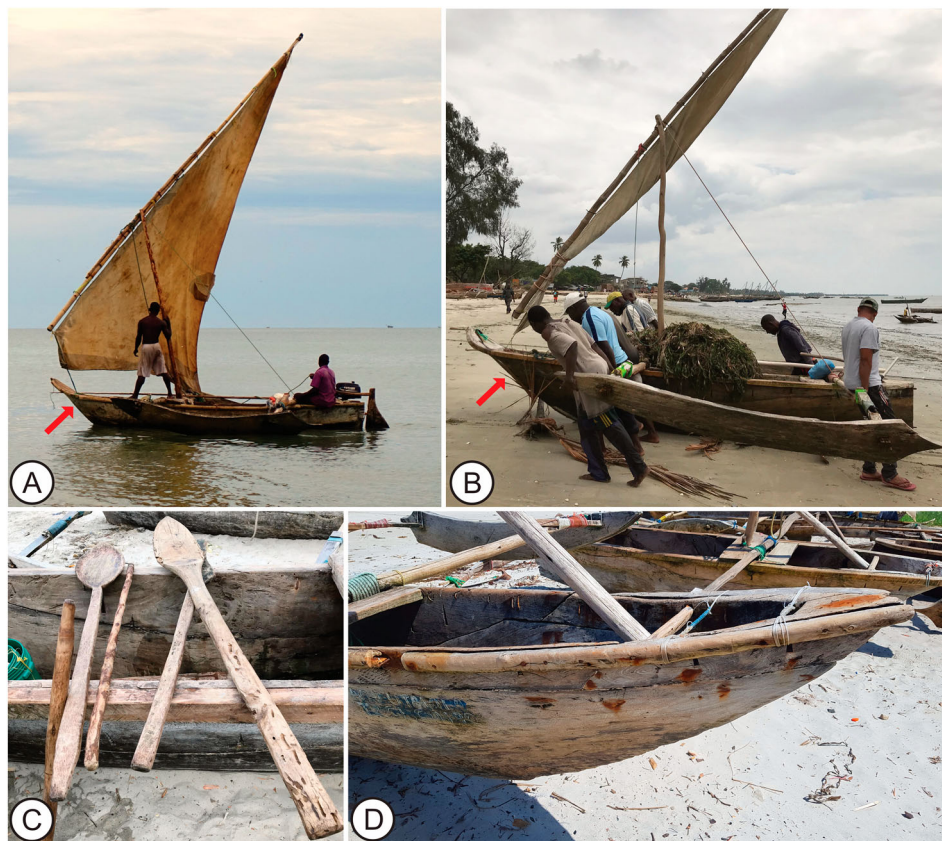
Figure 3. Ngalawas at Bagamoyo: (A) under sail in March 2020, with – unusually – an outboard motor as back-up; (B) crew and helpers hauling out after a fishing trip, August 2019; (C) ngalawa paddles, August 2019; (D) a hull lacking the ngalawa 's signature fore-wash-strake ( kasama ), February 2020. The red arrows indicate the lobed kasama bow timber (Images: John P. Cooper; Lucy Blue).
