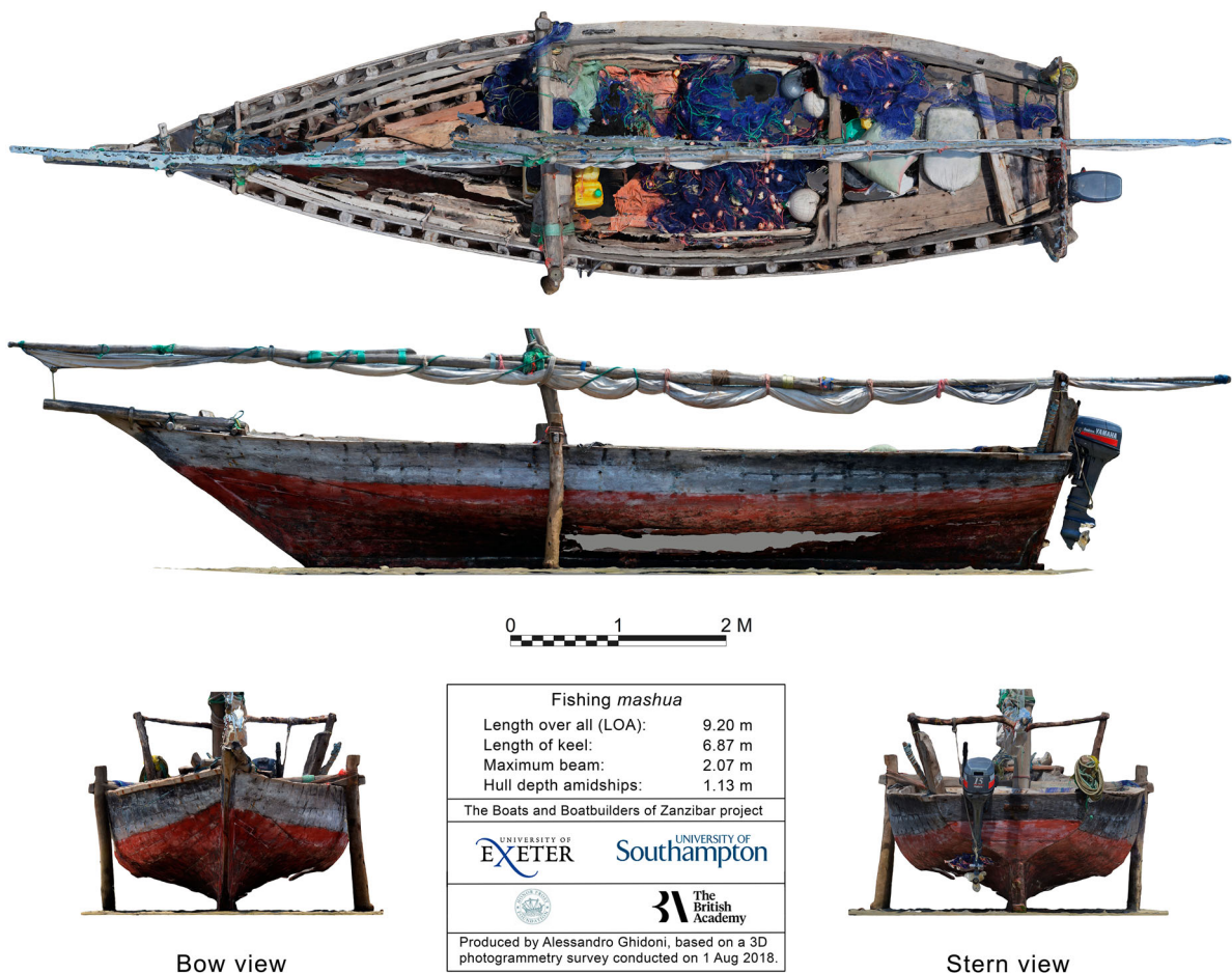
Figure 16. Orthographic views of a transom-sterned, plank-built mashua fishing boat, recorded at Mkokotoni, Unguja, in August 2018, based on a 3D photogrammetry survey (Image: John P. Cooper and Alessandro Ghidoni).
