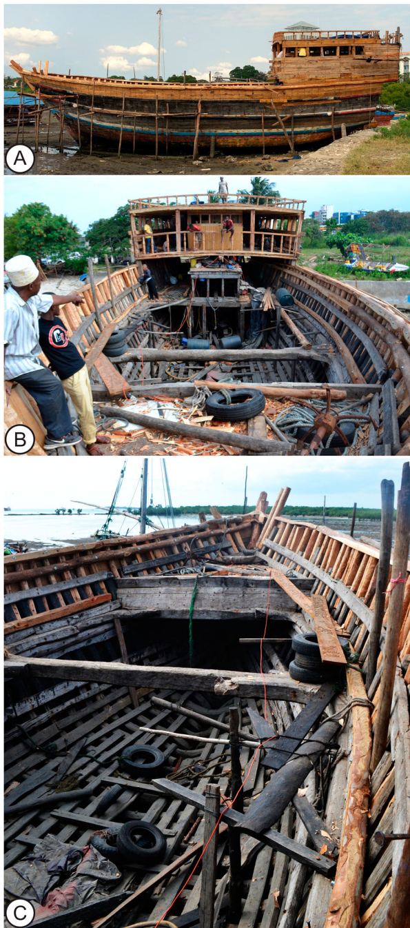
Figure 26. A cargo bumu having its sheer line extended at Kinazini, Unguja, August 2018 (Images: John P. Cooper and Alessandro Ghidoni).
