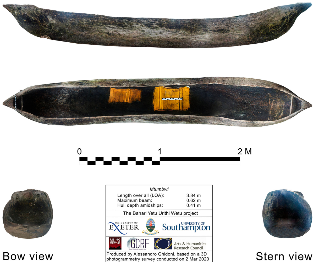
Figure 7. Orthographic views of a Lake Nyasa mtumbwi recorded at Bagamoyo in March 2020, based on a 3D photogrammetry survey (Image: Makanani Bell, John P. Cooper and Alessandro Ghidoni).
