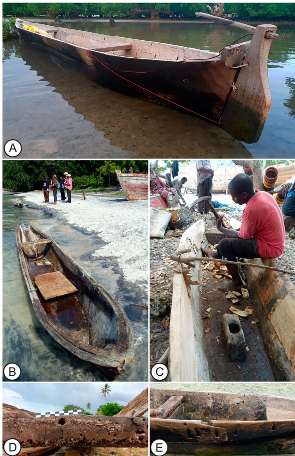
Figure 5. Mtumbwi construction features: (A) A recently completed 12 m-long vessel at Bagamoyo, March 2020, with a mast step and lateen rig stored inside, and a small wooden plate forward of the rudder indicating it can also take an outboard motor; (B) note the flat bottom and 'false' inner stem and stern features on this mtumbwi at Mlingotini, August 2019; (C) a carver at Marahubi, Unguja, trims a new extension plank while repairing a mtumbwi , July 2018; (D) the c.60 mm-thick base of a broken mtumbwi at Kaole, August 2019—note the dowel hole; (E) 'stitching nails' used to affix the extension planks to the base, Marahubi, Unguja, August 2019 (Images: John P. Cooper).
