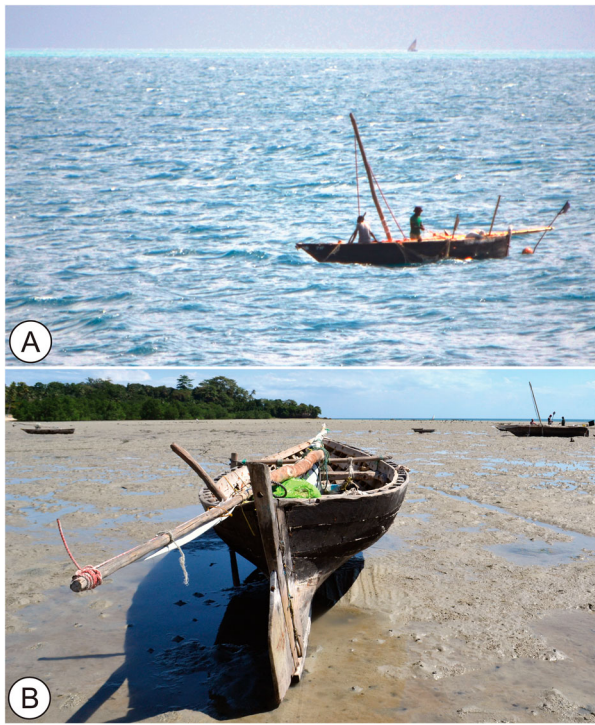
Figure 15. The double-ended mchoro fishing boat: (A) crew setting their nets near Stone Town, Unguja; (B) propped in the intertidal zone, Mazazini, Unguja (Images: Alessandro Ghidoni).
