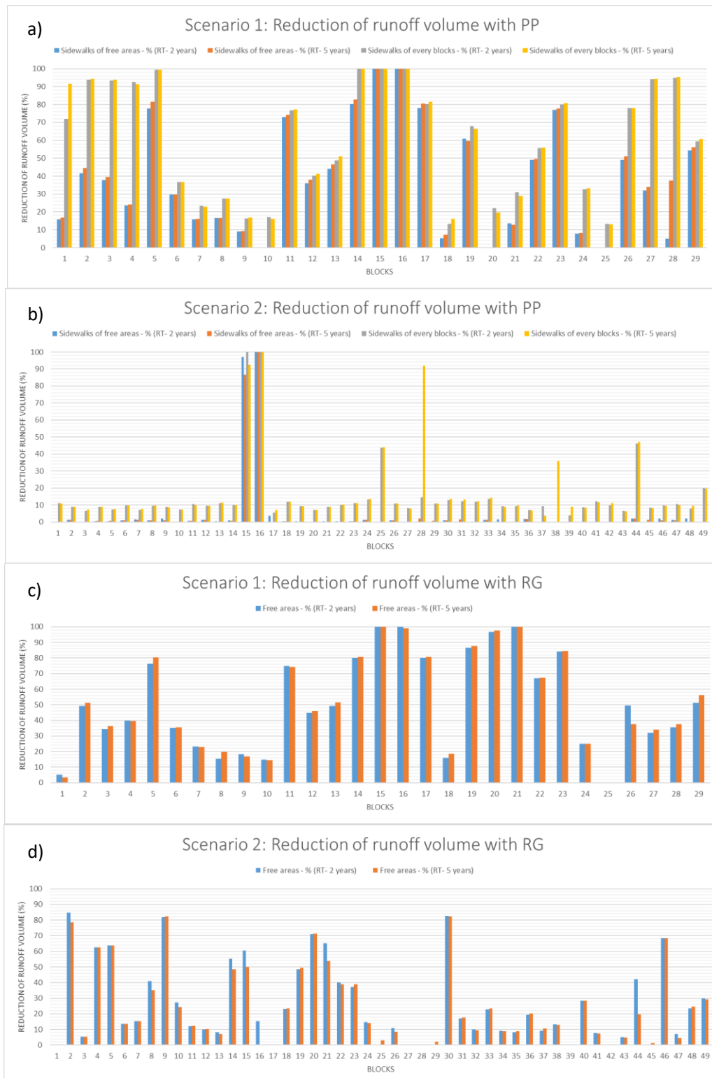
Figure E1. a) Percentage of runoff volume reductions with PP application in scenario 1, b) Percentage of runoff volume reductions with PP application in scenario 2, c) Percentage of runoff volume reductions with RG application in scenario 1, d) Percentage of runoff volume reductions with RG application in scenario 2.
