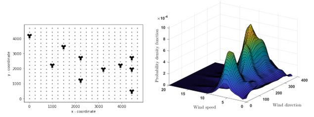
**Figure 2: Visual representation of the binary encoding (left). The 1s are the location of turbines and 0s are the empty space. Probability density function of the joint distribution of wind speed (m/sec) and wind direction (right).**
