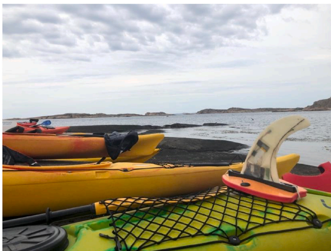
Fig. 6. Adaptation of the Smartfin for other watercraft (in this case, a sea kayak) by the fastening of a surf fin box to a small flotation device which is towed behind with a rope.
