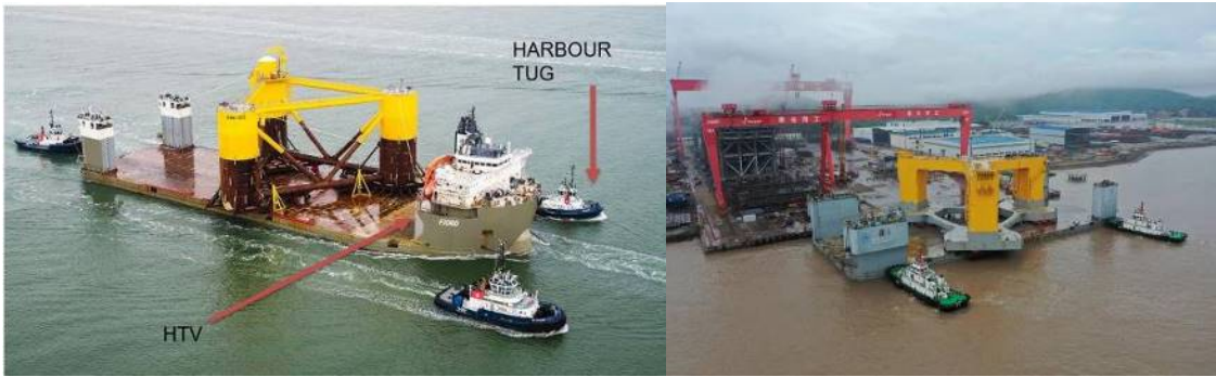
Figure 4 Dry transport of semi-submersible, ref [11] and ref[12]
