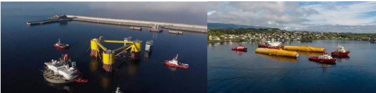
Figure 5 Floatoff of semi-submersible, ref [11], and Spar ref [8]
