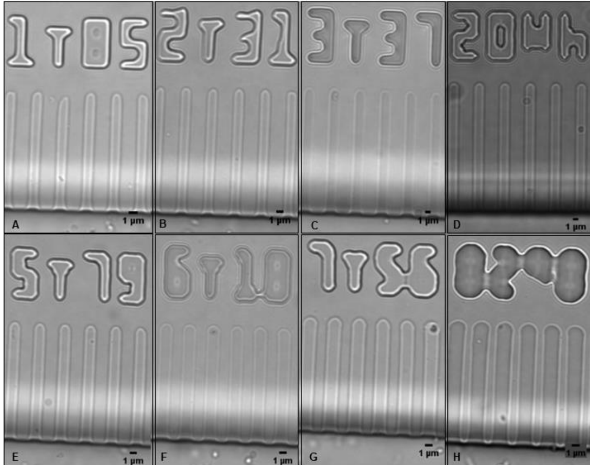
Figure 18. Different arms within the Modified Mother Machine under the microscope with a magnification of \times 100 . Width of the arms increase from A to G. As observed bacteria ( A, E ) and Ostreococcus tauri ( C, D, F, G ). It is noticeable the presence of certain forms that could be by-products or either bacteria or algae in early stages of development ( B, H ). All images were taken at t=0 immediately after seeding the device.
