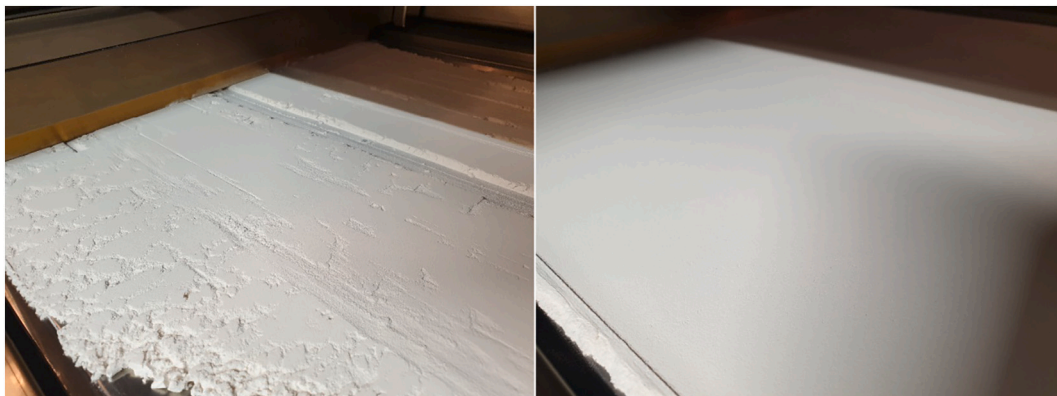
Fig. 2. Image of spreading trial fail result for PDK12 (left) and PDK12-T pass result (right).
