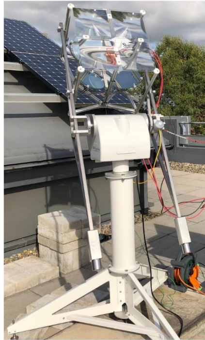
Figure 10 The integration of counterbalance arm, counterbalance weight, and UHCPV system to the sun tracker, where a. is the SOLIDWORKS design and b. is the full actual system outdoor ready for testing. The drawings in Figure 10a includes the extended tube but not the heavy-duty floor stand tripod, where Figure b shows the real heavy-duty floor stand tripod.
