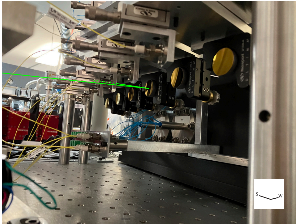
Figure 10. (Top) Schematic view of the fiber injection mount. CHARA beams are reflected by a gold coated off-axis parabola and focused onto a fiber tip. (Bottom) View of the six fiber injection modules for the AIO combiner mode, hanging from mounting plate. Four additional fiber injection modules for the ABCD combiner mode are mounted on a plate above (see far right side of Fig 8).
