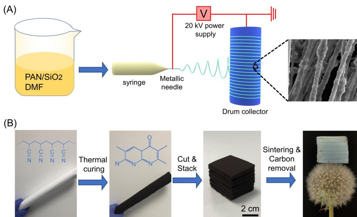
**Figure 2** (A) Schematics of the transformation of the PAN/SiO<sub>2</sub> nanofibre sponge to SiCNW sponge; (B-D) SEM images of the cross-sectional area of SiCNW sponge, the boundary between two adjacent layers is indicated by the arrows; (E) TEM image (inset is the SAED pattern); (F) TEM images of a SiCNW and the corresponding elemental maps of Si, C, and O; and (G) XRD profile of SiCNW.
