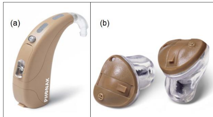
Fig. 2.6 (a) A body worn HA/BTE device [53] and (b) A RTE HA [71].
