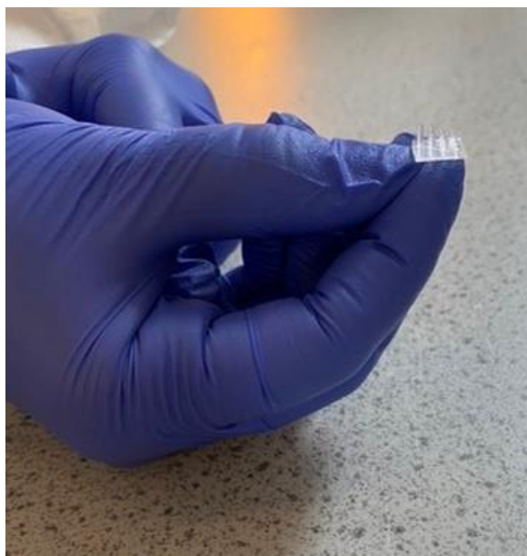
Fig. 4.7 The PDMS micropillars peeled off the SU-8 mould, from the UV method.
