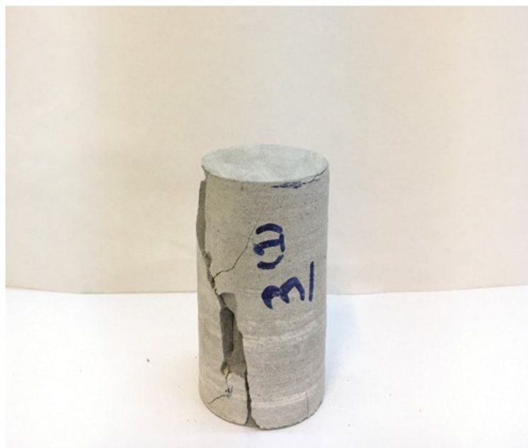
Figure 4. A sample of failure mechanism of UCS test.
