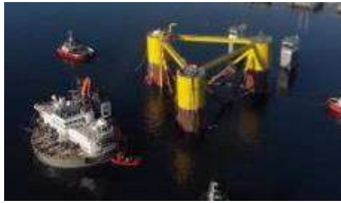
Figure 9 Semi submersible floatoff from HTV (Principlepower website, 2022)
