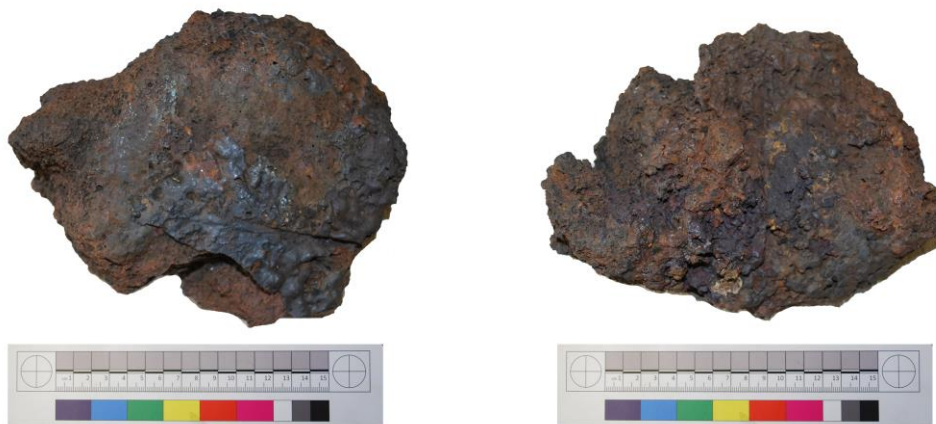
Figure 4.29. Dish-shaped hearth cake, displaying molten slag covering a rough top surface (left) and coarse underside showing debris impression (right). Note the rounded edges and a lateral protrusion, which could be an occluded slag channel.
