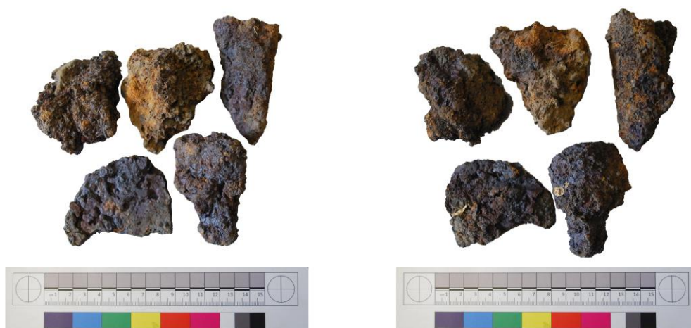
Figure 4.25. Example of iron-rich slag, showing rough purple surfaces. Note the plate and cone-shaped pieces, as well as the presence of adhering orange clay.
