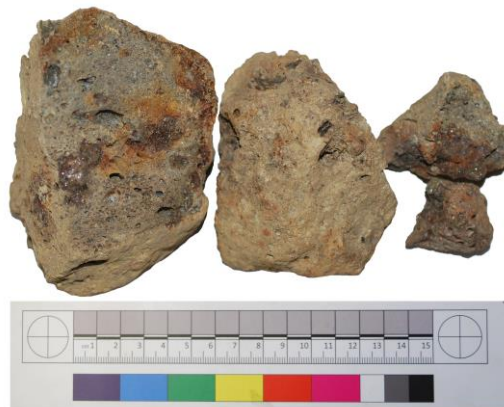
Figure 4.44. Examples of subtype II, showing a concrete-like appearance and vesicular interior. Note the brown and orange patches of iron.
