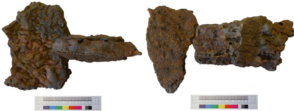
Figure 4.9. Tap slag cake weighing 13.5kg from QN1. Note the plano-convex shape and rounded edges of the fragment to the left. On the right the other fragment displaying in profile multiple flows of slag. Also, note the sandy rough underside. Top and bottom images are shown in Appendix A.1.1.
