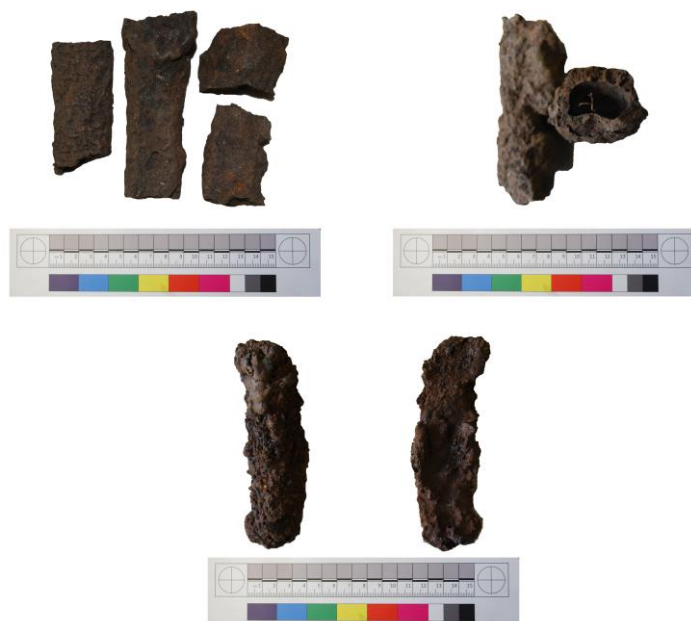
Figure 4.34. Examples of cylindrical rod of slag. Note the hollow cross-section and shape (top). Bottom: example of rod with flat top. Note the rough texture.
