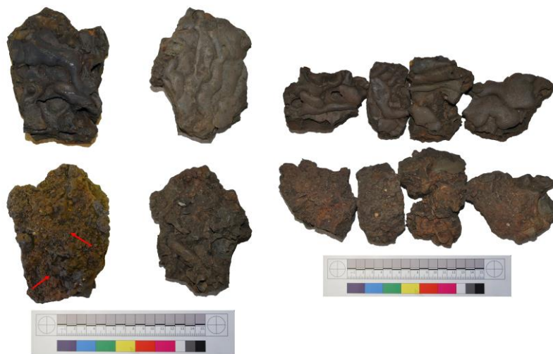
Figure 4.8. Left: detail of a fragment of tap slag cake, showing the underside with many charcoal (red arrows) and angular stones impressions. Right: Broken fragments of tap slag cakes, whose top and bottom surfaces are preserved. Note the orange clay adhering to the underside.
