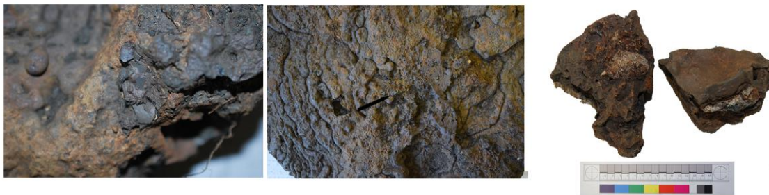
Figure 4.13. Details of tapped slag cakes, showing possible hammer scale attached to the bottom surface (left), a prill of metal in the centre of the cake (left), and fragments with possible blast furnace slag inclusions (right).
