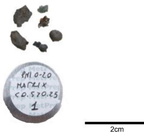
Figure 5.15. Selected sample matrix from trench PN1 0-20 (sieved through <0.50\text{cm}>0.25\text{cm} ) including two fragments of flake hammerscale, spheroid hammerscale, a small green fragment of blast furnace slag (top) and iron-rich slag fragments.
