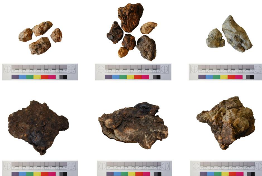
Figure 4.48. Top: small clay fragments showing signs of burning. Colours vary from pink (left) to yellow and dark orange (right) and light grey (left). Bottom: largest piece of hearth bottom displaying a thick layer of slag and iron on the top surface (left), in profile (middle) and on the underside (right) shows the same clay colours observed in the small fragments, some of which may derive from larger hearth lining pieces.
