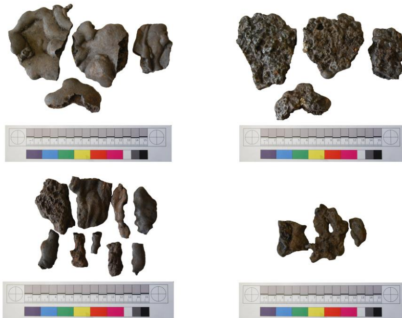
Figure 4.20. Top: examples of slag plates displaying flow pattern on top and undulated undersides. Bottom: slag tendrils, also including possible slag prills. Their undersides show ground debris impressions (bottom right).
