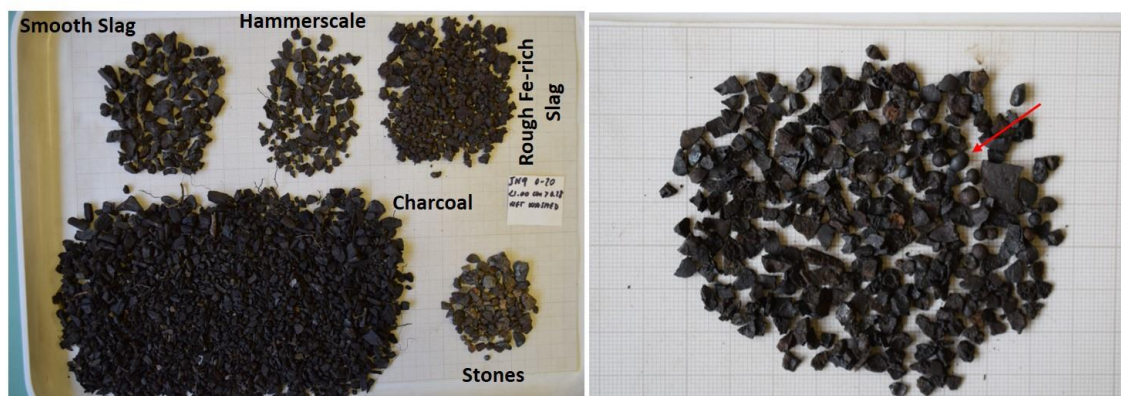
Figure 4.51. Matrix material from trench JN9, which contained the largest amount of this type of slag (left). Right: Hammerscale from the same trench, both flakes and spheroids (red arrow) are present.
