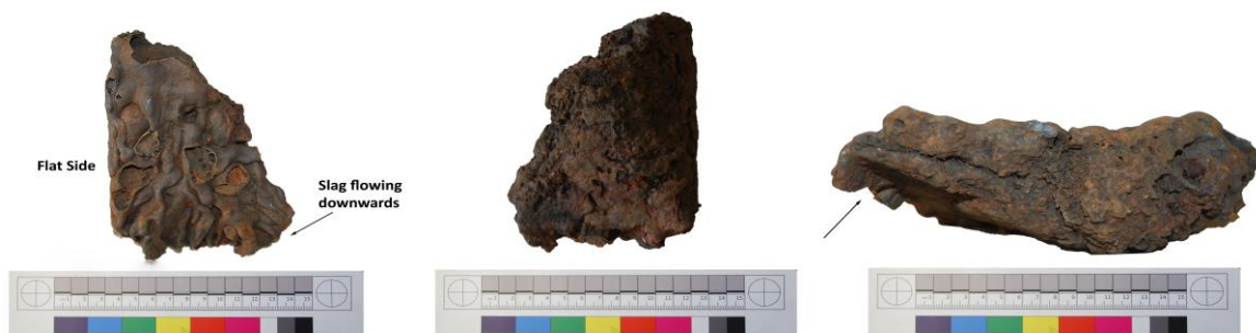
Figure 4.10. Example of tap slag cake from ZS3 (20-40) which displays a flat side (left and centre) and slag flowing downwards following the profile of what were presumably the edges of the hearth installation (right). The picture in the centre shows the underside.
