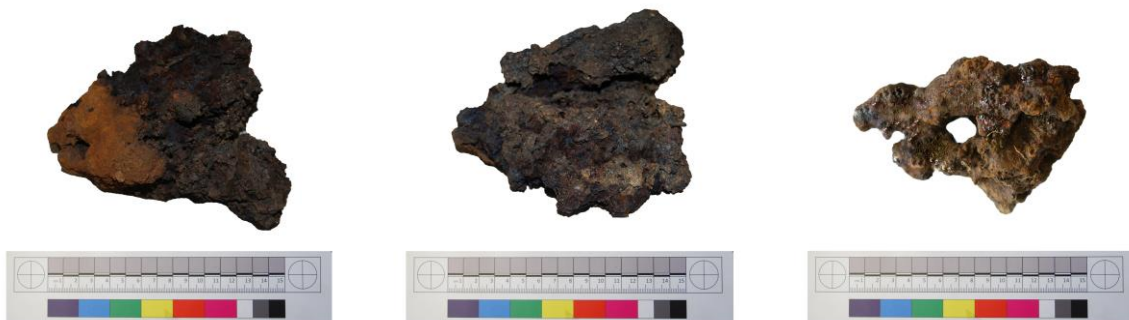
Figure 4.26. Left: slag with clay attached to one end and hole running through the body of the piece. Centre: detail of the back of the slag showing the length of the cavity. Right: ring of slag, the piece is characterised by a rough texture and feels sandy to the touch.
