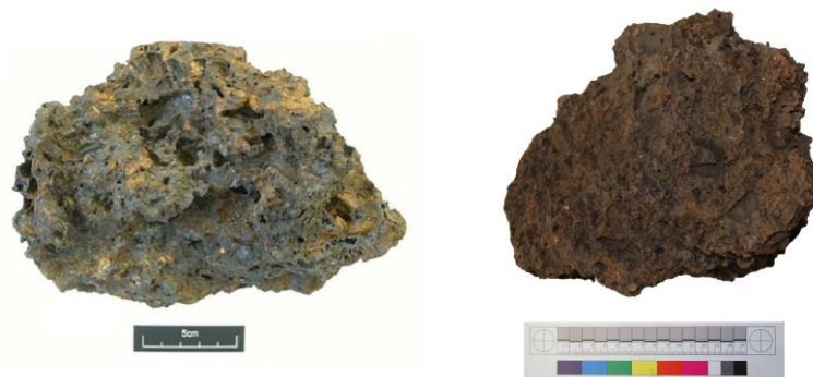
Figure 4.2. Comparison between an example of furnace slag produced from bloomery smelting and excavated from a Late Iron Age site in Kent (left) and an example of hearth slag from Ausewell Wood. Note the coarse texture and small charcoal impressions (photo on the left after Girbal 2013, fig.9, p.96).
