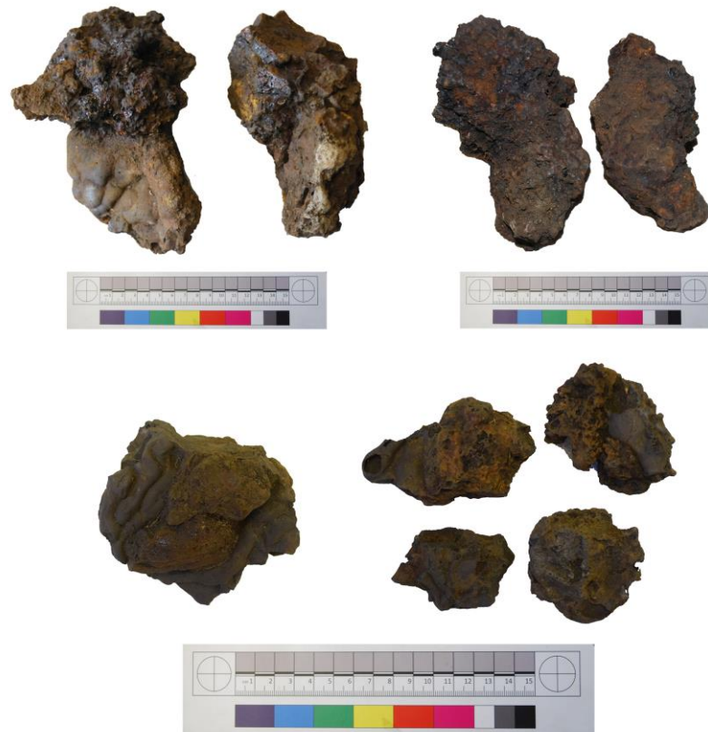
Figure 4.15. Examples of mixed rough/tap slag. Note the globular protrusions of rough slag on top of the smooth flowing slag. All pieces display iron-rich areas.
