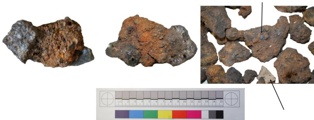
Figure 4.28. Details of slaggy conglomeration pieces, showing blue and black blast furnace inclusions. Also note the white stone inclusion, the small pebbles and sand particles. All pieces show some degree of vitrification.
