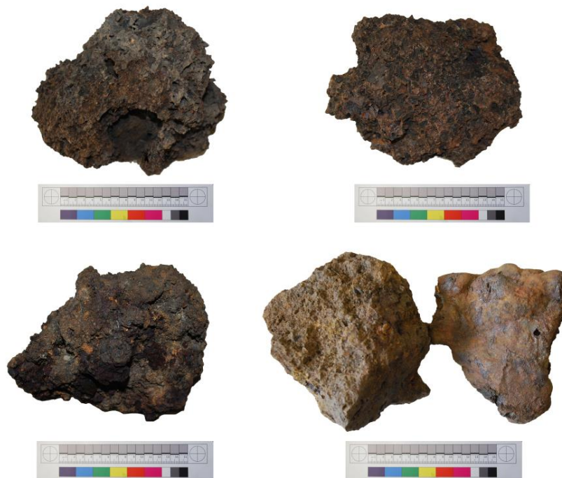
Figure 4.32. Saucer-shaped example of hearth slag, displaying a pointy slag protrusion on the underside (top). A possible typical example of 'hambone' is shown on the bottom. Note the orange clay and iron-rich areas visible on both pieces.
