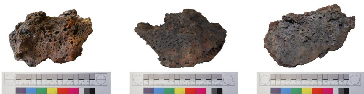
Figure 4.31. Examples of hearth slag cakes on profile. Porosity becomes progressively larger towards the upper layers. Note the bowl shape of the piece in the middle, with an extended rim and slag accumulation on top.
