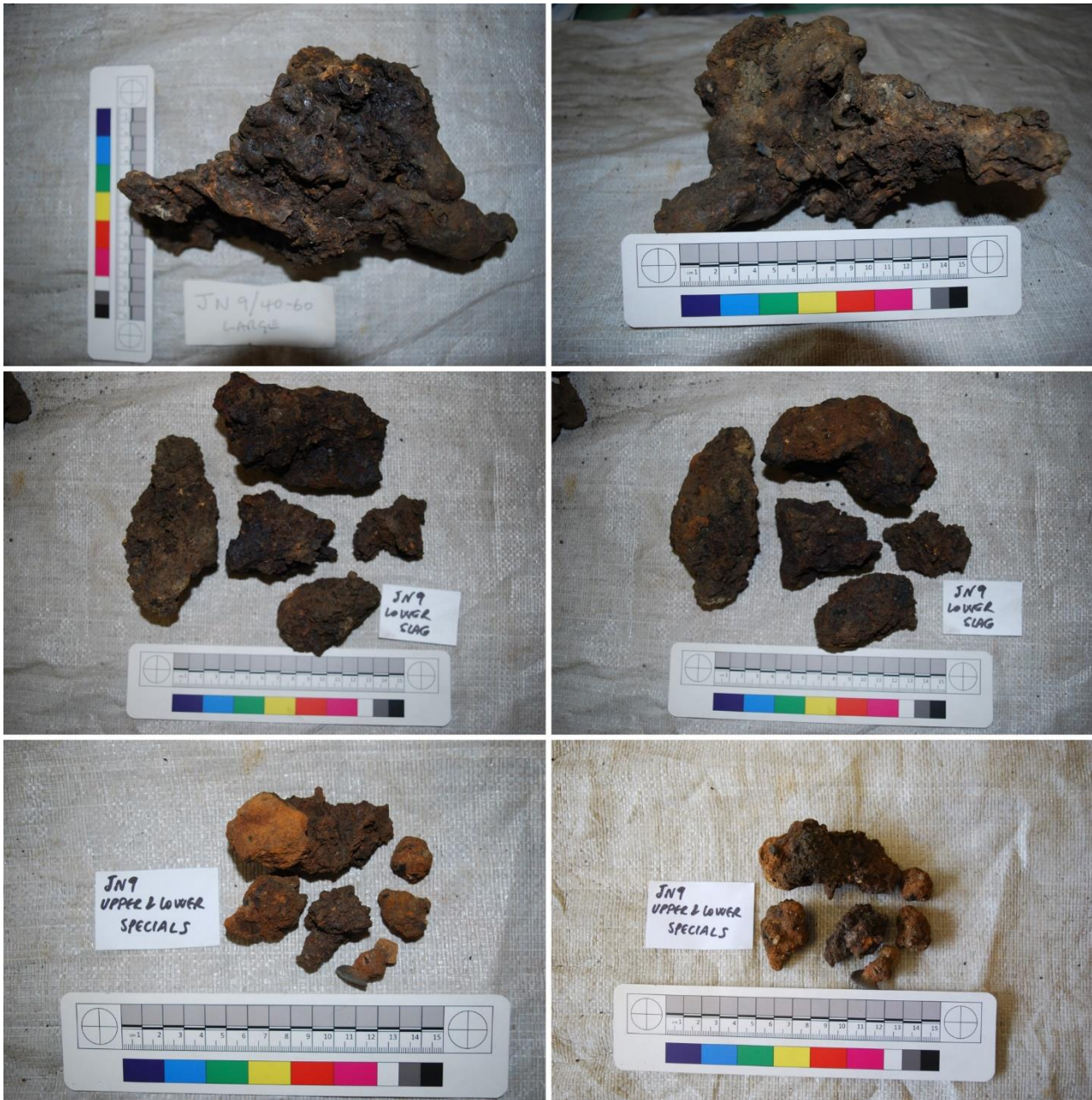
Example of material debris recovered from trench JN9. Located 9m away from the baseline excavation, the material in this trench appears characterised by iron-rich fragments and several slag channels fragments (section 4.4.2).
