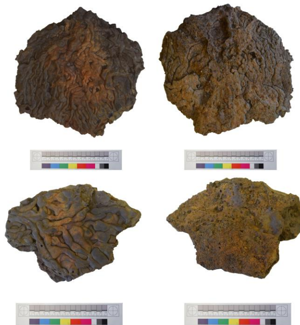
Figure 4.7. Tap slag cakes (QN1 0-20) showing the typical flow pattern on top surfaces (left) and underside with ground debris impressions and rough textures (right). Note the plano-convex shape and rounded edges.
