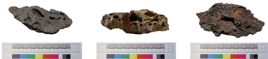
Figure 4.18. Side profile of three examples of flowed cakes from trench ZS3. Larger spherical voids are concentrated on top surfaces, with smaller rounded porosity towards the upper layers. Example on the right is showing at the centre a rectangular cavity left by a slag channel.
