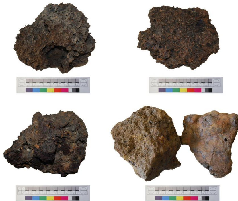
Figure 4.30. Examples of hearth slag cakes and blocks. Numerous charcoal inclusions and impression characterise their surfaces. Note the slag channel visible on the centre of the piece on the top right. Examples that derive from JN9 display some different features. The piece on the bottom left, while of a similar texture, is rich in iron; also note the small slag protrusion on the top left. To the bottom left, two blocks of a smoother texture, with molten slag and charcoal inclusions.
