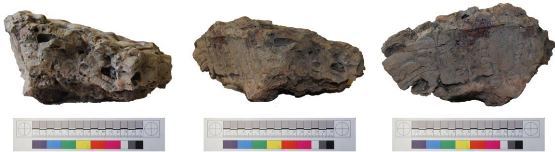
Figure 4.11. Example of tap slag cake from ZS3 (20-40) showing a flat smooth profile, which becomes thinner as the slag flow runs perpendicular to the side. Also note the purple patches of iron.
