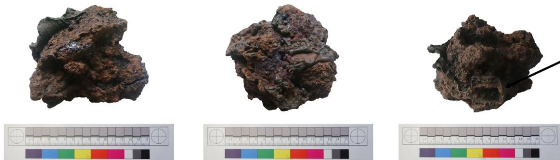
Figure 4.19. Slag cake found in ZS3 (0-20), showing features in between rough and tap slag (top). Note the molten slag on the underside (bottom left). Bottom right: side profile showing a rectangular section of a possible slag channel. Refer to the slag channels described in the text.
