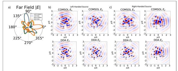
**Figure 7.** Comparison between our analytic results, based on the discrete dipole approximation, and full-wave simulations in COMSOL. Considering only the 20 (of 64) scatterers nearest to the source of the device shown in figure 3 of the main paper, we compare (a) the far-fields and (b) and (c) the near-fields. For these scatterers, 65 nm radius silicon spheres, good agreement with the discrete dipole approximation is shown.
