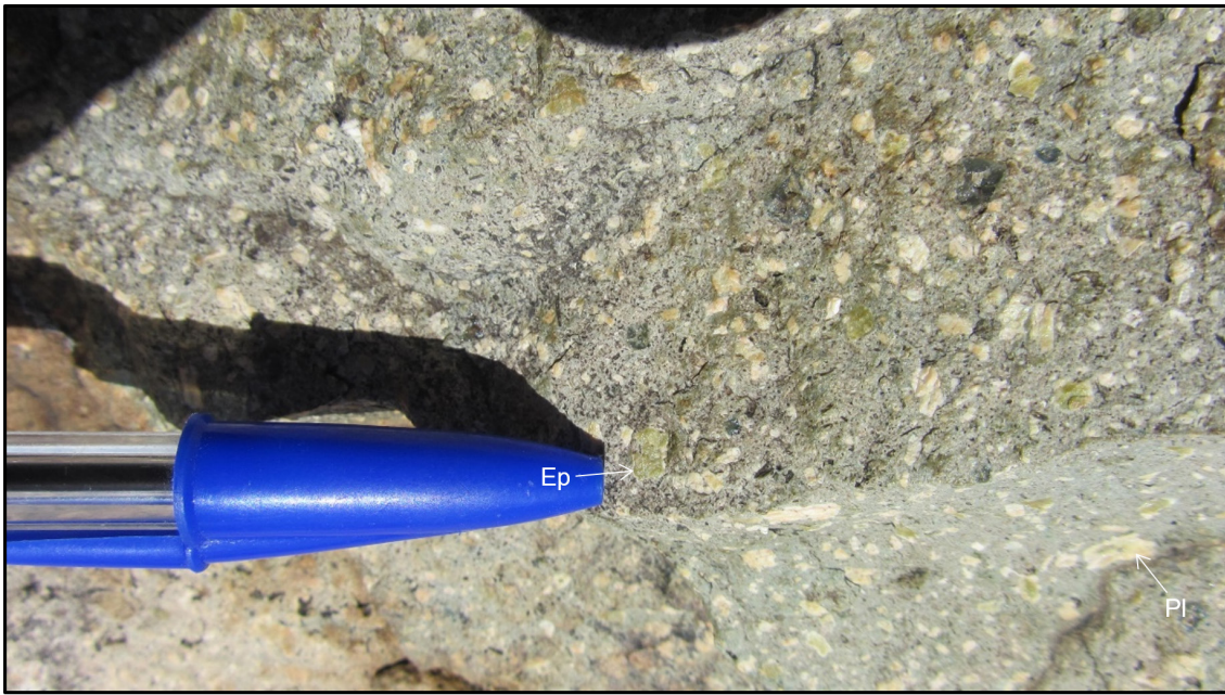
Sup. fig. 5.7 Propylitic alteration in Fulstone Spring Volcanics: which overlie the Yerington porphyry system (Dilles, 1987). Epidote (apple green; Ep) is seen replacing primary plagioclase (milky white; Pl). Pen for scale. Zircon LA-ICP-MS trace element data for this sample (BS10) is presented in Fig. 5.7 .
