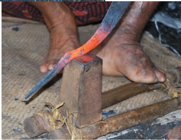
Figure 6.10 Shaping the tip (left). Using the large hammer as an anvil and shaping a bend in the sickle (right).
