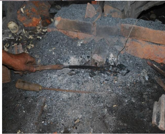
Figure 6.5 Burying the object in the dirt during heat treating (left) and moving object just over the fire during heat treating (right).
