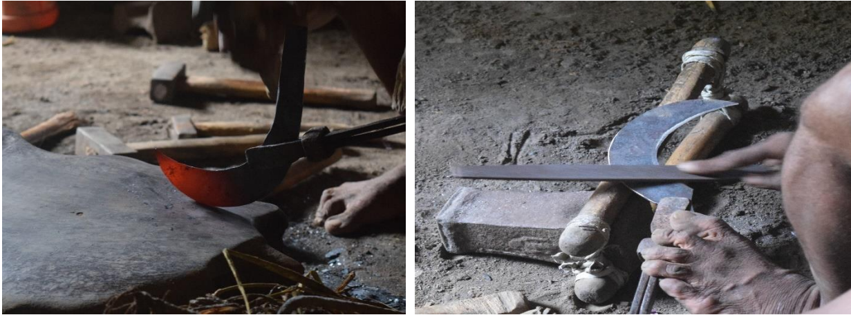
Figure 6.15 Forging the tip of the blade (left), sharpening the blade (right).
