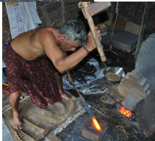
Figure 6.18 Preparing to use the large hammer during forging (left) and using the large hammer to forge the handle (left).
