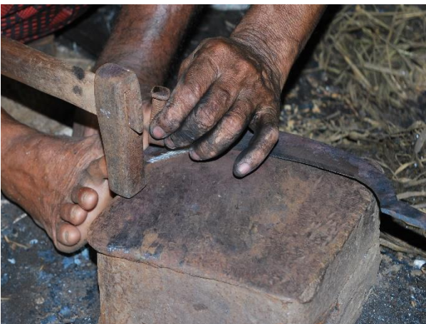
Figure 6.11 Using a small chisel and hammer to make small marks along the blade.
