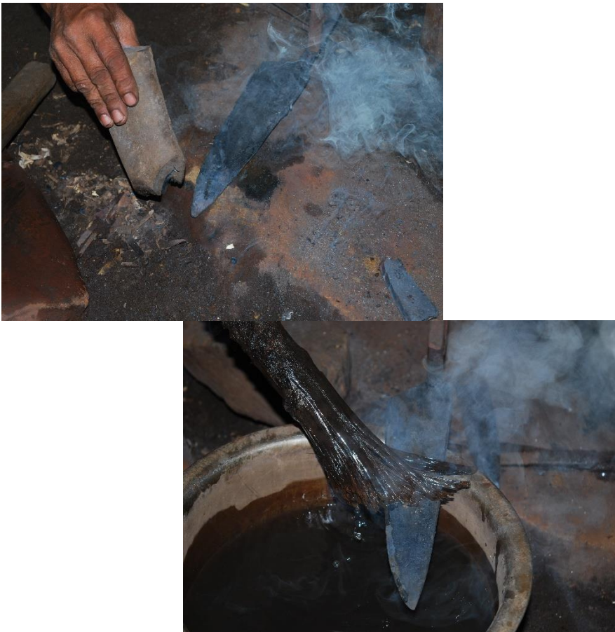
Figure 6.2 Using bull horn to make the iron mild (left). Using the frayed stick soaked in water for heat-treating (right).
