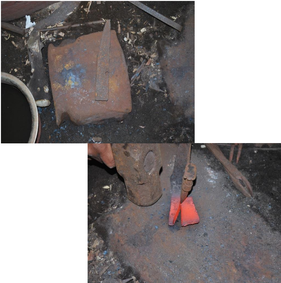
Figure 6.1 Starting piece of scrap (left). Cutting unwanted pieces off the object (right).
