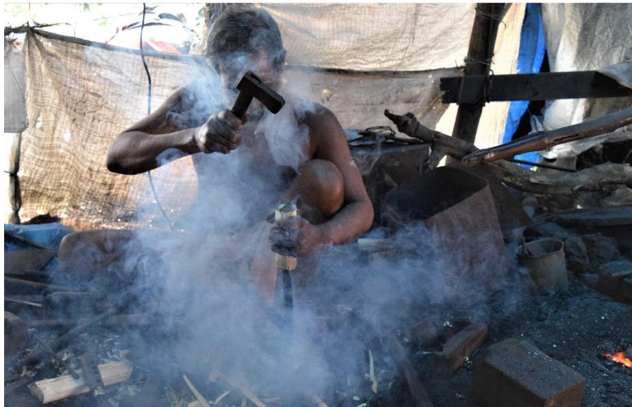
Figure 1.1 Premanath T.N. in his forge in Vypin adding a wooden handle to a knife (Edwards 2017).
