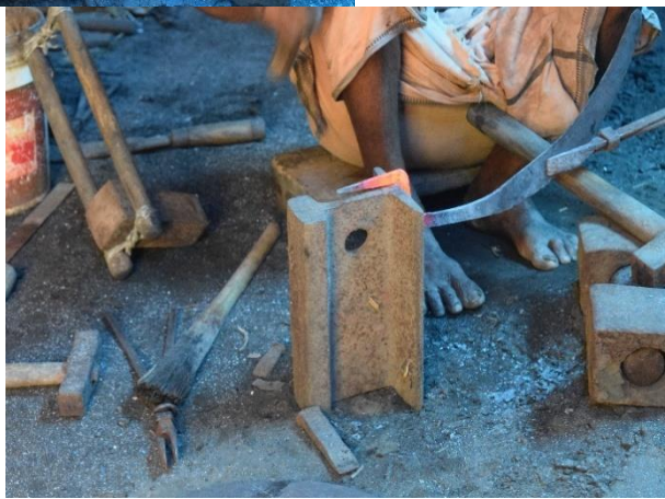
Figure 6.21 Drawing out the tang while forging (left). Creating the curve in the handle (right).
