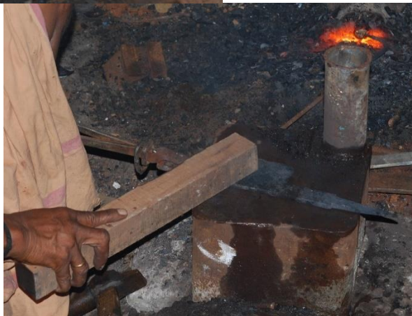
Figure 6.7 Using iron tool and hammer to shape tang (left). Rubbing a wooden block on the object to make the iron mild (right).
