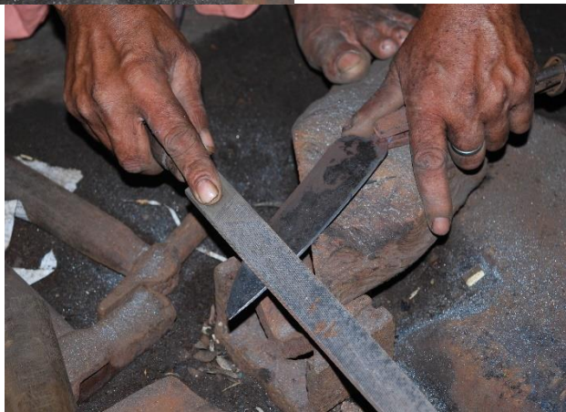
Figure 6.4 Shaping and spreading the blade section (left) and sharpening the blade with a hand file (right).
