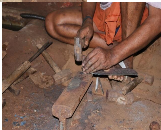
Figure 6.13 Dipping the blade into water during heat treating (left) and using a punch to make a hole in the handle (right).
