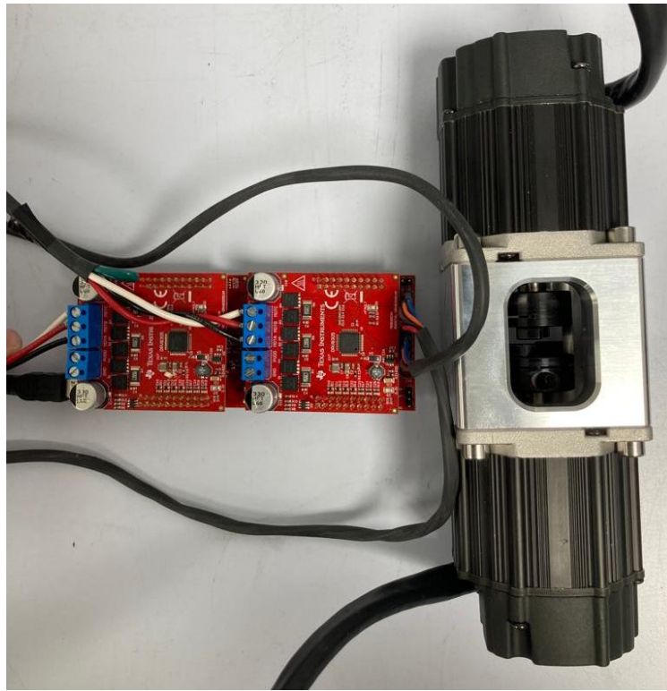
Fig.5.10. Dual motor coupling and LAUNCHPADXL controller
