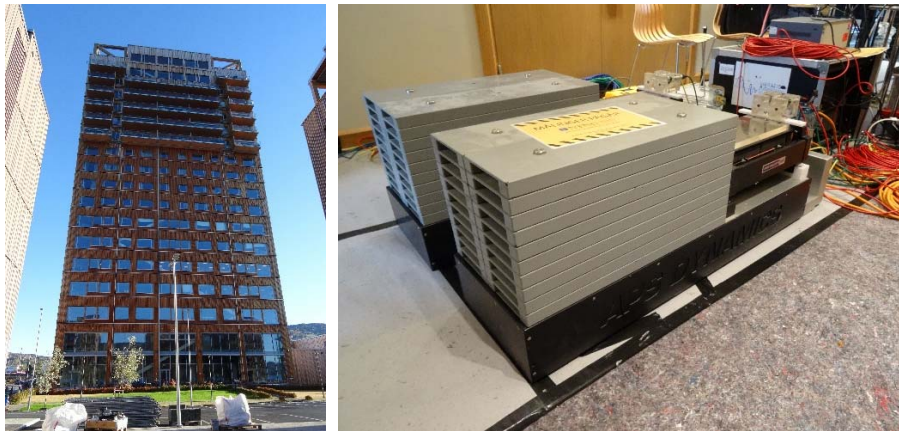
Figure 36: Photo of the application of APS shaker with horizontal reaction mass system.
