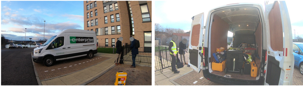
Figure 19: A long wheelbase van with equipment packed and ready to be deployed. The total weight of the equipment was less than 1 tonne and individual pieces were less than 50 kg each enabling safe and easy manual handling by two people.
