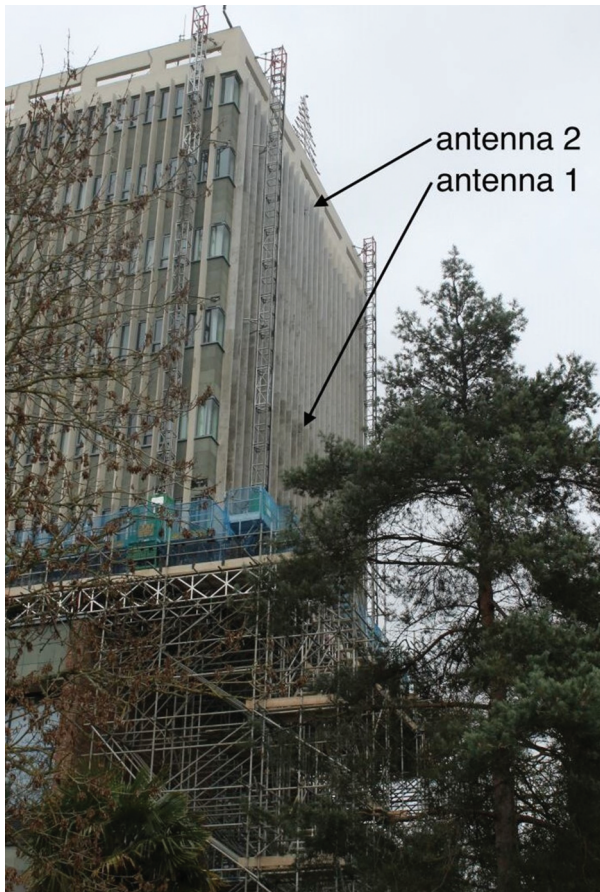
Figure 3. Experimental two-element interferometer deployed on the physics building at the university of Exeter.
