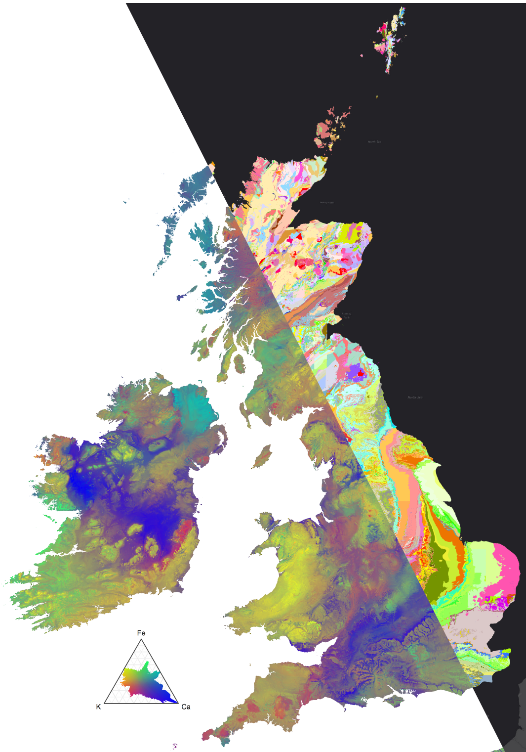
Figure 7.6: (Left of diagonal) AI-generated ‘properties first’ geological map, which provides probabilistic predictions of geological properties through space. The properties mapped here are centred log-ratios of potassium (K; red), iron (Fe; green), and calcium (Ca; blue) concentrations as observed in stream sediments. (Right of diagonal) A traditional ‘classification first’ geological map whereby rock units are manually classified according to convention. Source: The British Geological Survey’s Geology of Britain Viewer ( http://mapapps.bgs.ac.uk/geologyofbritain3d/ ). Contains British Geological Survey materials © UKRI 2022
