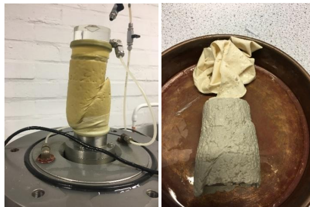
Figure 3.14 Sheared triaxial samples.
