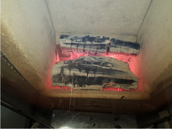
(c) Run 3, event d - collapsed logs
