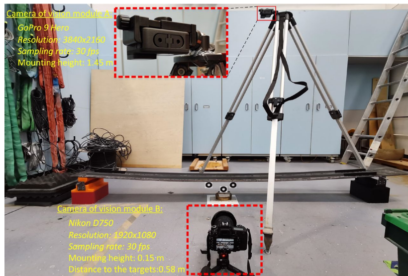
Fig.7 Layout of cameras for vehicle tracking and structural displacement measurement
