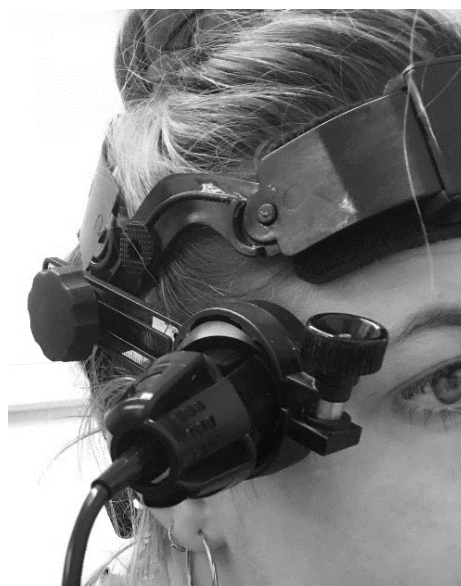
Figure 3.2 Transcranial Doppler ultrasound secured in place using an adjustable headset to measure cerebral artery blood velocity during the neurovascular coupling and cognitive function tests.
