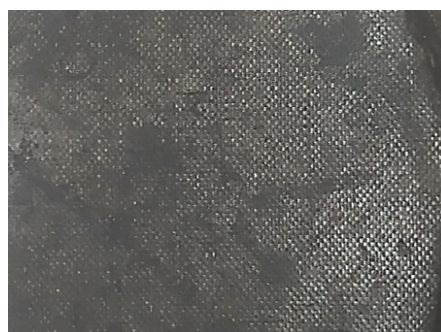
Figure 4.7: Digital camera image of nylon fabric coated with FLG flakes, following the dip and dry method.
