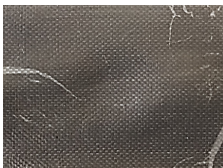
Figure 4.9: Digital camera image of nylon fabric coated with FLG flakes, following membrane dip coat method.
