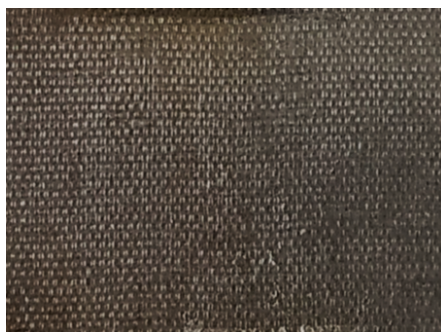
Figure 4.12: Digital camera image of nylon fabric coated with FLG flakes, following ultrasonic spray coating method.
