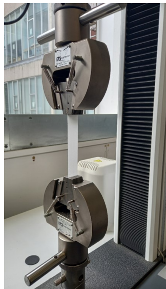
Figure 3.15: Instron 3367 static tensile tester loaded with the polyester fabric of 15 cm × 2.5 cm dimension, clamped tightly with 2716-015 manual wedge action grips.
