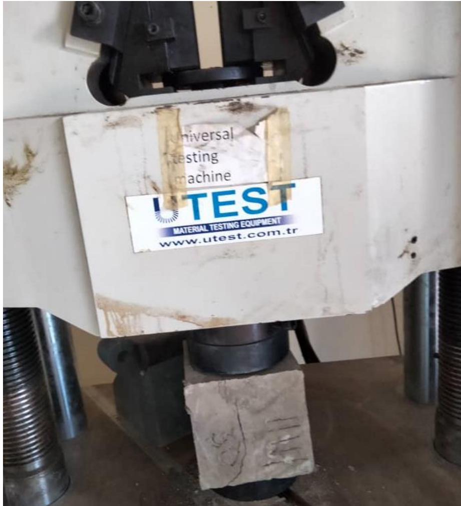
Fig. 3. Compressive strength test on sample cube
