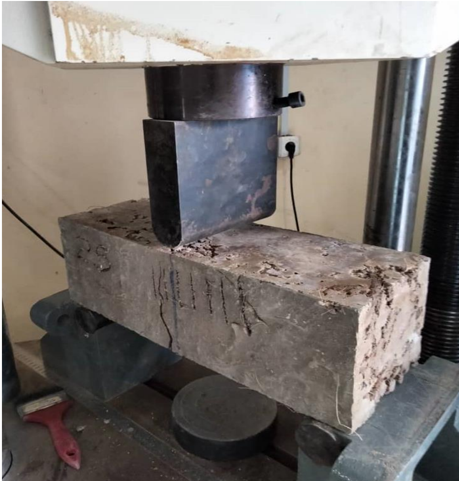
Fig. 4. Flexural strength test on sample beams
