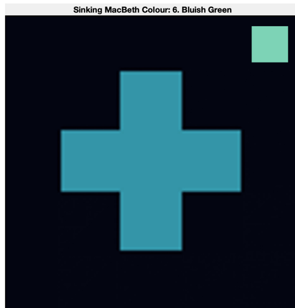
Fig. 1. Sunken cross-shaped object with Lambertian reflectance (dry colour displayed in top-right) at a depth of 2.5 m in chlorophyll-free water.
