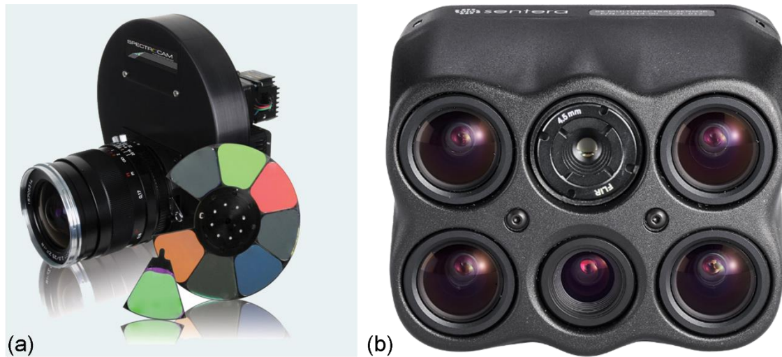
Figure 8: Example configurations of multispectral imaging systems, multiple interchangeable filters [77] (left) and multiple filter/lens/sensor units [78] (right)
