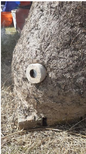
Figure 4.76 - Left a tuyere embedded in the wall of an experimental bloomery furnace. Right, a Sri Lankan tuyere made of fired clay. The Tudeley accounts record how the tuyeres were made of iron. (Author's images).
