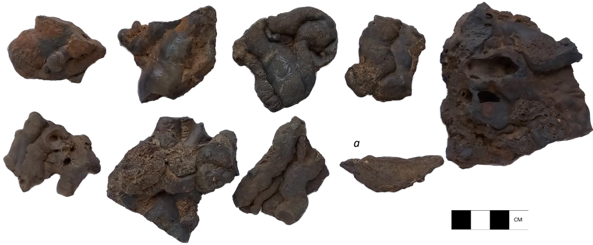
Figure 4.89 - Examples of Type 2 slag recovered from Roffey. Many of the examples only showed 2-3 flows, unlike the large cakes of slag at Tudeley. They would suggest that like the experimental smelt, tap slag was removed from the tapping pit during the smelt, preventing the formation of large slag cakes. Slag 'a' appears to retain the lower edge of the hole made by the boring stick and like Type 3 slag, solidified in the hole. (Author's image).
