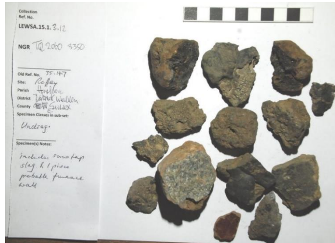
Figure 3.14 - slag (including tap slag) and probable furnace wall recovered by Straker in his visit to Roffey in the 1930s. Now held in the Straker collection at Barbican House. Image courtesy of www.slagdata.org
