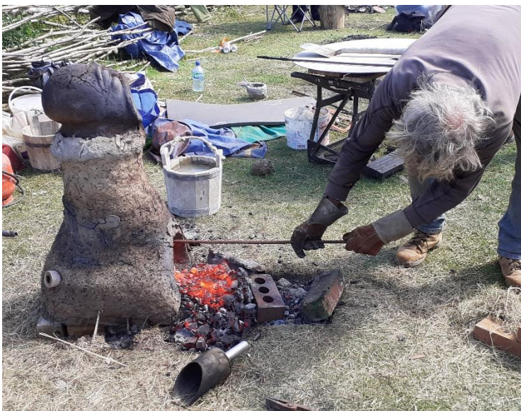
Figure 4.78 - Raking out the furnace through the tapping arch to remove the bloom along with slag that has solidified within the furnace. At Roffey this furnace slag was classified as Types 1 and 4. (Author's image).
