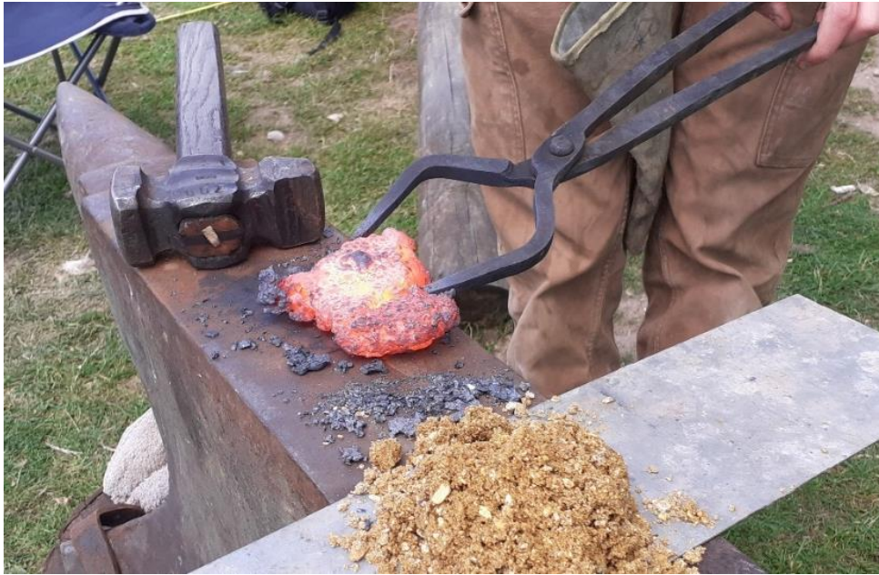
Figure 4.82 - Consolidating the bloom into workable iron through a combination of heating and hammering. Slag can be seen around the consolidated bloom, having flaked, or been driven off during the hammering. (Author's image).
