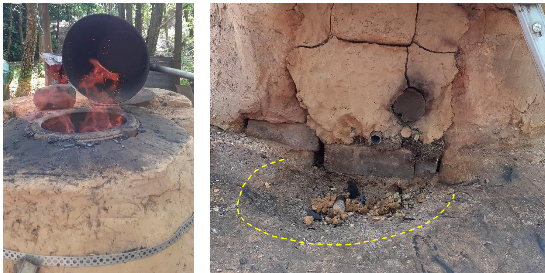
Figure 4.84 - The furnace is charged with ore and charcoal. At the base of the furnace the tapping arch is blocked with clay and a small pit to catch tapped slag dug adjacent to the arch (yellow). This pit collects the early runs of tap slag (Type 2) that escape through cracks in the tapping arch. (Author's image).
