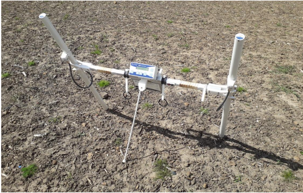
Figure 2.11 – Bartington Fluxgate Gradiometer Grad601r used at both Tudeley and Roffey. (Authors image)
