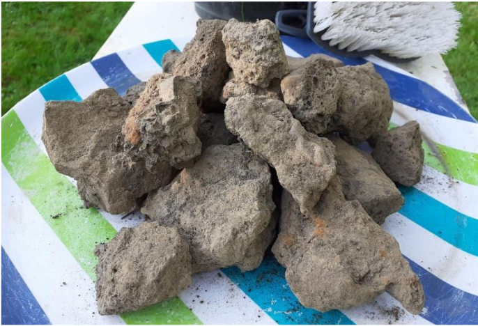
Figure 4.26 (left) - Unwashed slag. While washing all the slag took considerable time, the morphological characterisation of the slag was reliant on identifying characteristics such as colour, porosity, impressions, and inclusions, that could not otherwise be determined from the mud covering the slag. (Author's image).
