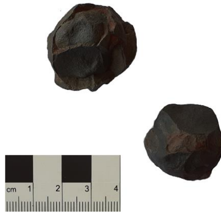
Figure 3.61 – Siderite ore recovered in Zone 1 at Cherry Tree Field. Fieldwalking revealed consistently-sized fractured samples c.2.5cm, some of which had a high magnetism, suggesting it had been roasted. (Author's image).
