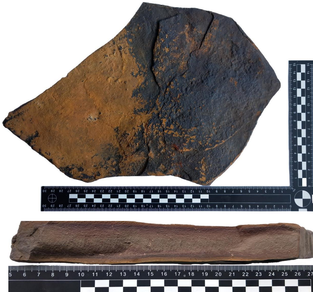
Figure 6.39 –Fractured fragment of the seam of siderite ore exposed on the western bank of the stream, below a layer of Wadhurst clay. This piece had been eroded out of the bank and lay on the stream bed. It is likely that erosion of the stream bank and the resulting exposure of these seams first attracted the smelters or ore diggers to the locality, where they excavated the eastern bank to exploit the continuation of this ore. (Author’s Image).
