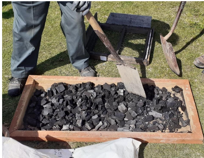
Figure 6.14 - Crushing the charcoal into a smaller charge. The sieve in the background was used to separate larger fragments for further processing. Sieves could also be used to separate the fines. (Author's image).
