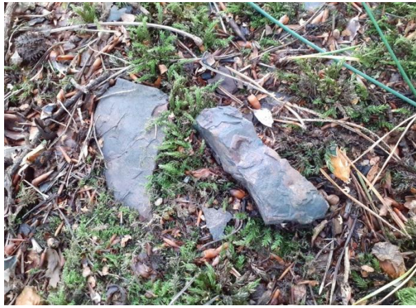
Figure 3.41 – siderite iron ore deposits found on an associated spoil heap adjacent to a minepit. Its thickness is indicative of the thin seams in which the ore is found. Pieces of sandstone, forming the waste rock or 'gangue' was also identified in these spoil heaps, but often formed small fragments of under 10cm. The larger rocks may have been removed if suitable for building material. (Author's image).
