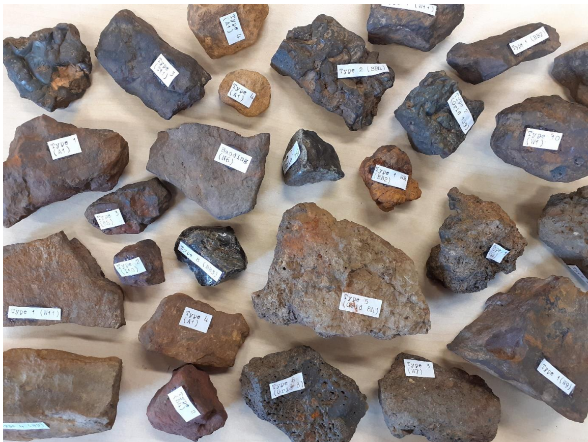
Figure 4.35 – A typological assemblage was created for slag and geological samples based on their morphology. They were labelled for easy reference. If a new type was identified that did not correspond to any existing sample in the collection, it was classified as an additional type and the sample added to the typological collection. A total of 10 types of slag were identified and 5 geological types. (Author's image).
