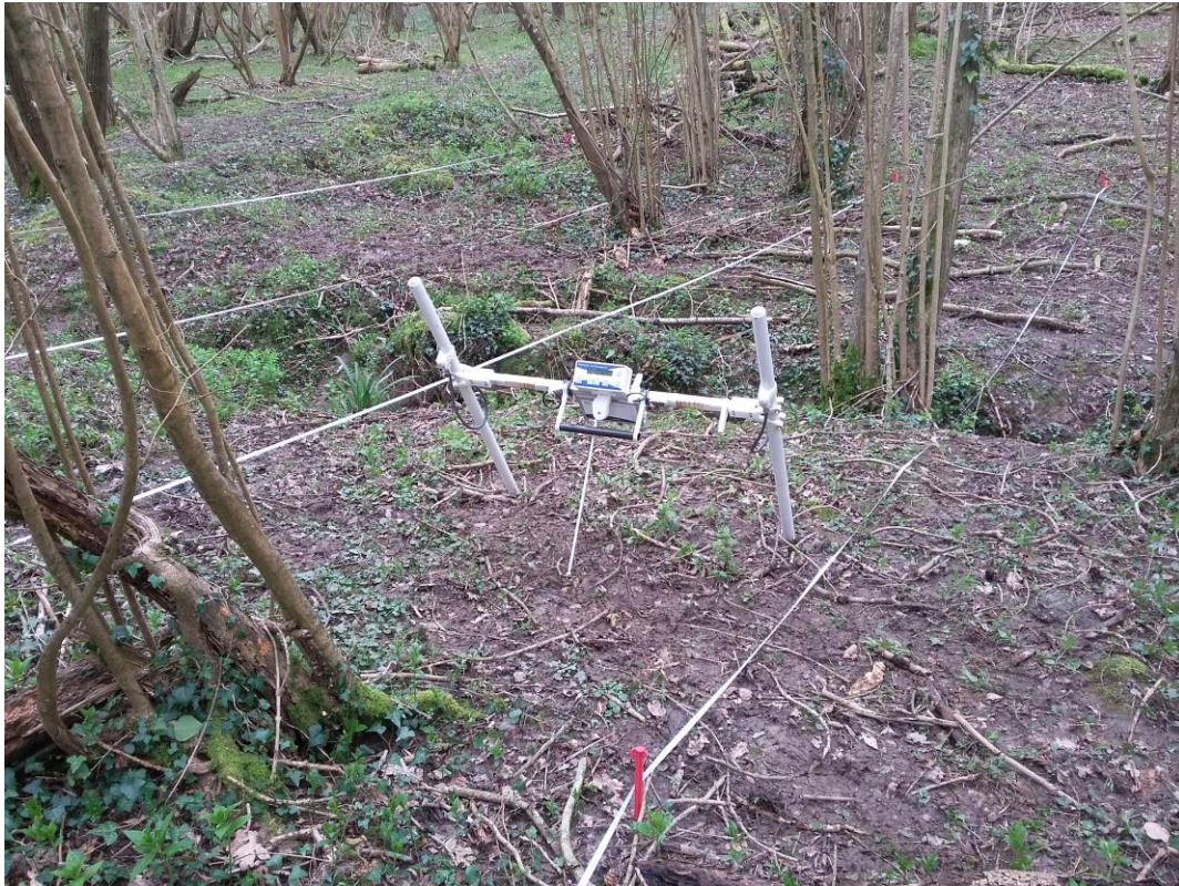
Figure 5.34 - The magnetometer took readings 0.5m either side of both sensors and meant each 10m grid was surveyed through 5 traverses on a parallel north-east alignment. Trees, vegetation, and the tributary stream meant that dummy readings had to be inputted within some traverses. To allow for the dummy readings a 'point plot' approach was taken, where readings were manually recorded every 25cm along the traverse demarcated by a tape measure. This meant 4 readings were taken per meter. The ability to input dummy readings was particularly important in grids 5-7 that covered the tributary stream and involved surveying as far as the southern edge of the stream channel, and walking around to the opposite bank (dummying out the appropriate number of readings) to continue to the end of the grid – a process that was particularly time consuming. Laying out tape measures along the traverse intervals of 1m, 3m, 5m, 7m and 9m, meant that readings could be accurately taken at 25cm intervals, totalling 40 readings per traverse, 200 readings per grid square and 3200 readings across the entirety of the site. (Author's image).
