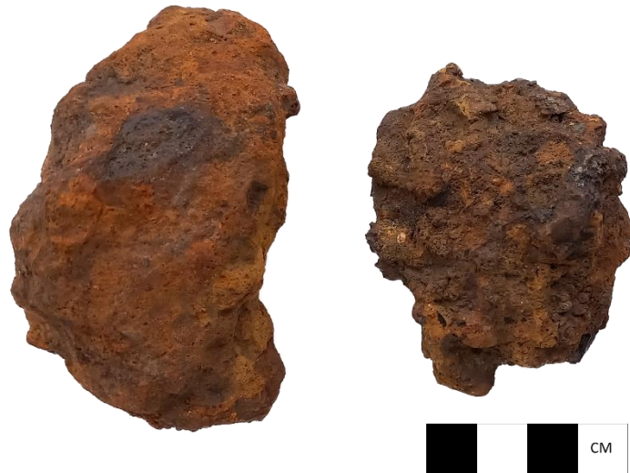
Figure 4.95 - The bloom is consolidated, and slag is driven off and build up within the hearth to form consolidation slag or primary smithing slag. This was recorded as Type 1 (WR) (right) at Roffey and constituted 6.10% of the assemblage. (Author's image).
