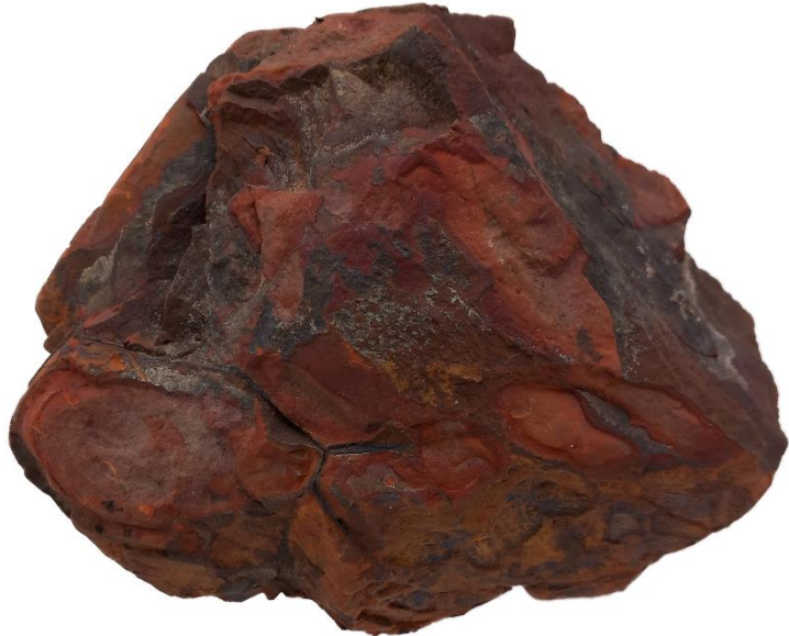
Figure 5.66 – Nodule of roasted siderite ore recovered amongst the slag deposits in the tributary stream. Its red to purple colour along with its fractured and friable outer surface indicate that it had been roasted. (Author's image).
