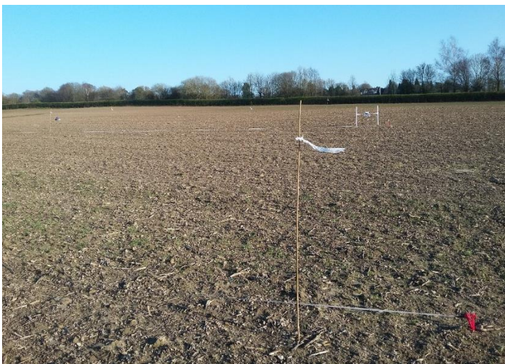
Figure 4.3 – Magnetometry grid. The 20m grid positions were marked with red tent pegs and tapes laid out at either end. A bamboo cane was placed at the end of each traverse to act as a guide. (Author's image).
