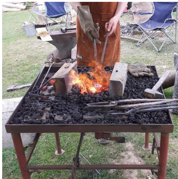
Figure 4.81 - Consolidation hearth or string hearth, used to re-heat the bloom prior to hammering in the primary smithing stage. (Author's image).
