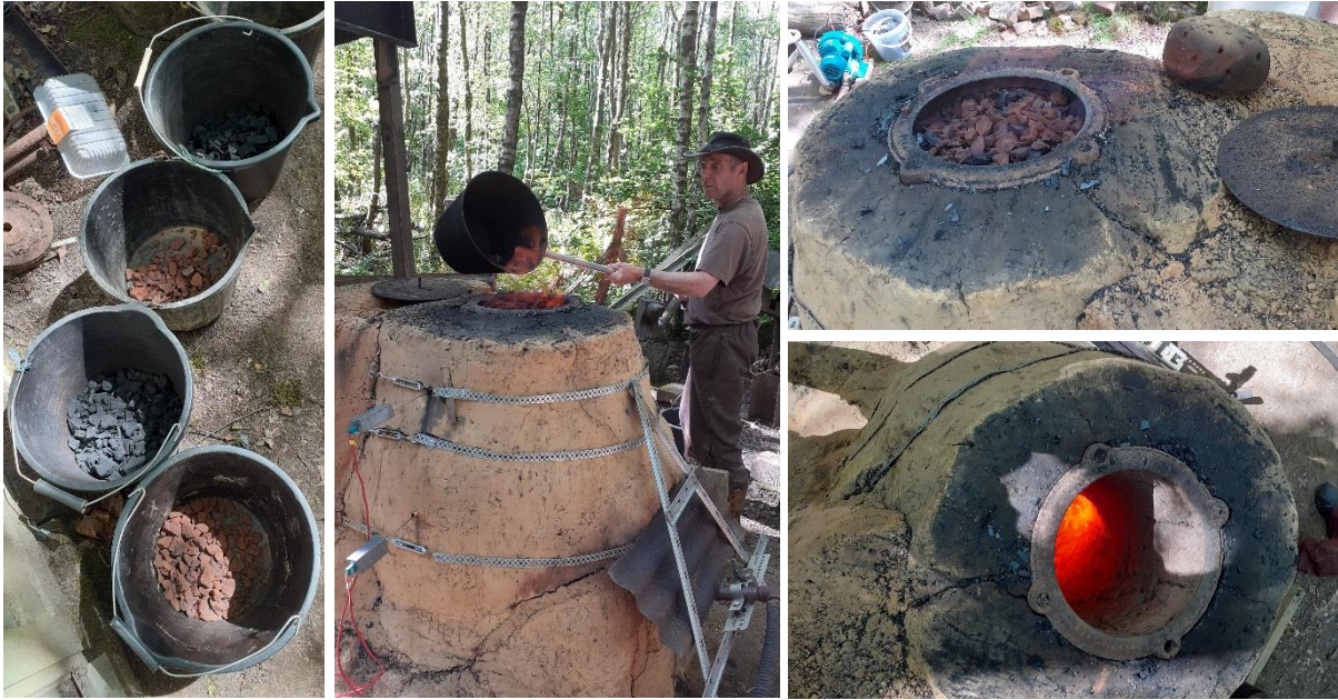
Figure 4.75- Charging the furnace – alternate loads of charcoal and prepared ore (possibly through roasting) are placed into the top of the furnace. The fuel to ore ratio is important. As the charcoal burns and the ore reduces, further charges are added. (Author's image).
