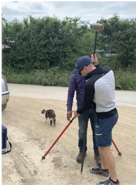
Figure 7 Collection of GPS data for CRL's gravity survey.
