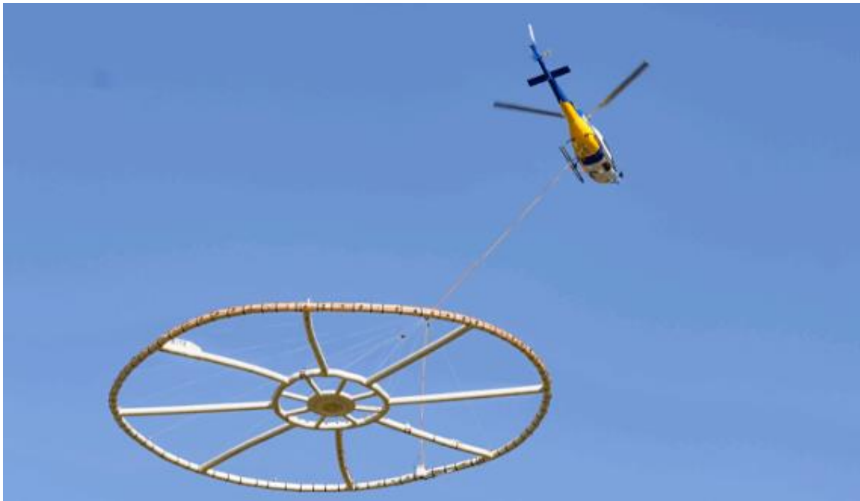
Figure 3 NRG Helicopter with towed sensor equipment
