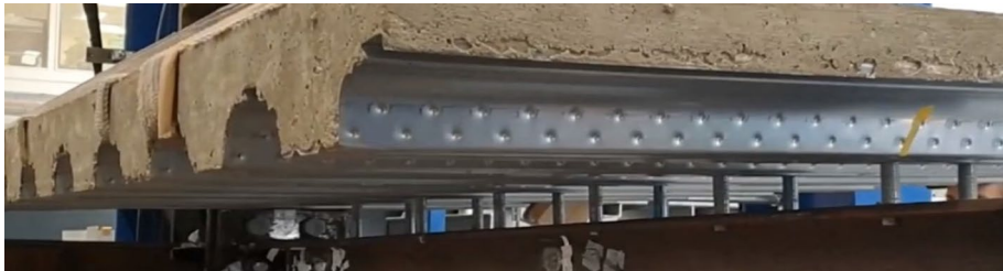
Fig. 13 Disconnecting the composite slab of the solid connection specimen to be reused for the next test
