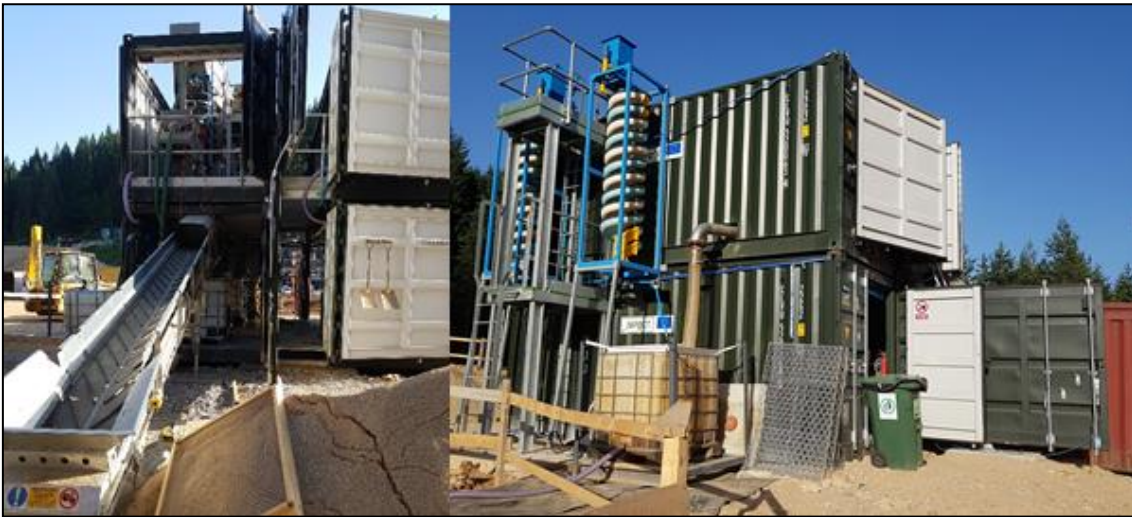
Figure 3.15: SOSO Mobile Modularised Plant comprising of four containers, developed by the University of Exeter. Left - Start of gravity beneficiation circuit. Right - External view of MMP.
