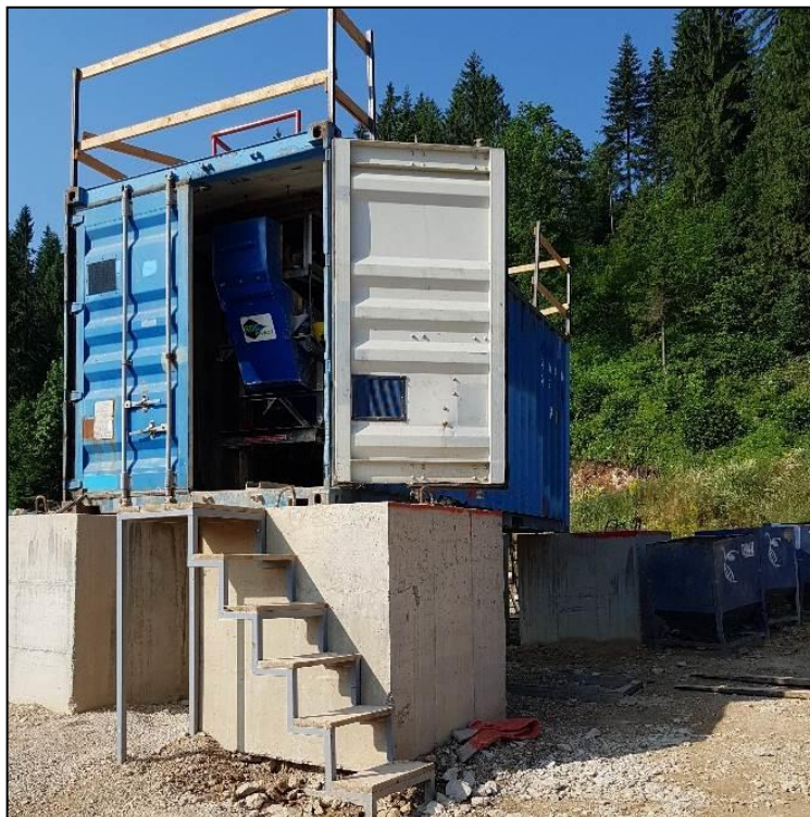
Figure 3.13: SOSO Comminution Module developed by Extracthive, set up for commissioning and testwork at Olovo.
