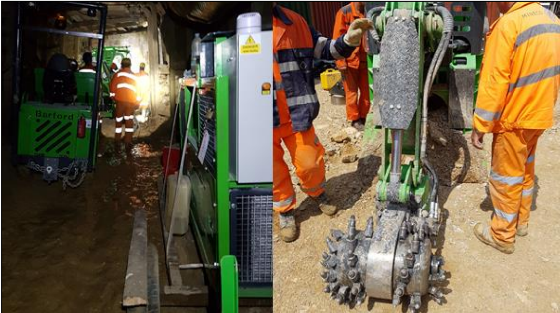
Figure 3.11: SOSO Selective Mining Tool developed by Metal Innovations. Left - Selective Miner, Dumper & Power Pack during Olovo testwork. Right - Selective Miner undergoing maintenance.
