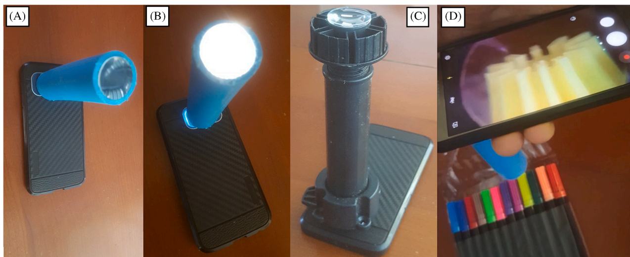
Fig. 5. A developed prototype smart fundoscope. A,B: Case attached with sterile plastic tube containing lenses. C: Screw prototype with adjustable lens height for focusing image. D: Example of the high magnification capabilities of proposed smart fundoscope.
