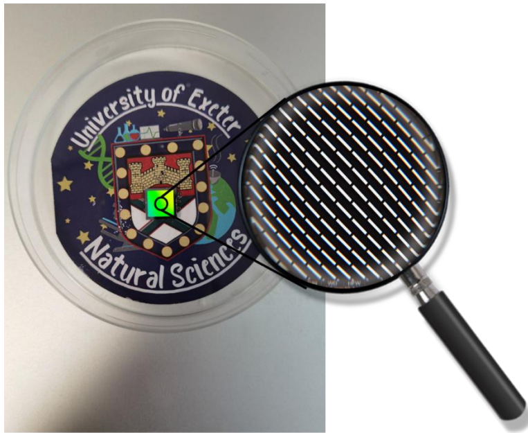
Figure 4.3 Images of the nanorod-based metasurface studied in this thesis. 1cm*1cm sample on Natural Sciences badge. Figure in magnifier is SEM image.
