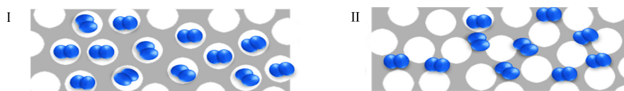
Figure 1. Two different types of diffusion can exist in a porous quantum system: (I) gas molecules (blue spheres) fully adsorbed within the pores. (II) Gas molecules diffuse through interstitial spaces due to the quantum effect.
