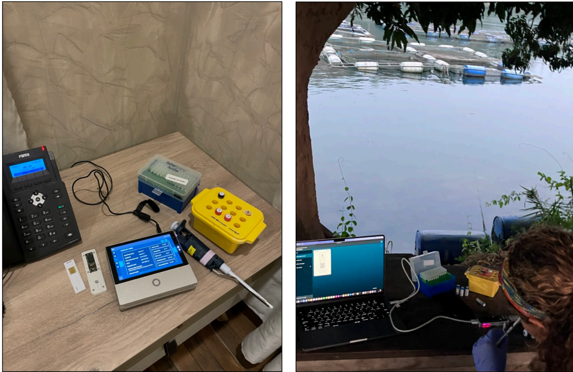
Figure 2. In-field sequencing, in a hotel and near the fish cages on Lake Volta, Ghana. Sequencing tissue samples using the MK-1C (ONT) on the left, and the MK-1B (ONT), on the right.
