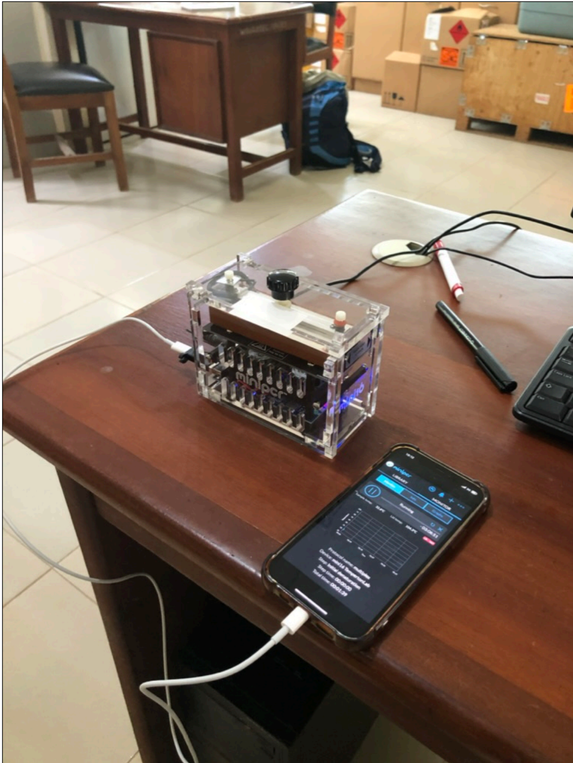
Figure 1. A MiniPCR machine connected to a mobile phone, performing a tiled PCR on ISKNV isolates collected from Lake Volta, Ghana.
