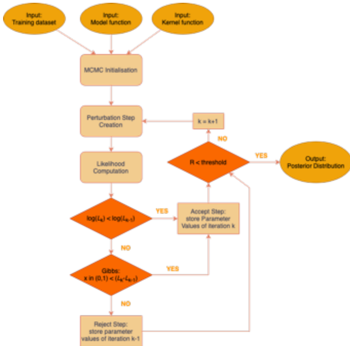
Figure 3.6: Flowchart representing the basic workflow of MCMC techniques. Inputs and outputs are represented by ovals. After MCMC initialisation, the algorithm goes through 5 basic steps which are iterated until convergence is reached: perturbation step creation, likelihood computation, likelihood comparison, step acceptance/rejection (with appropriate parameter storing), and convergence assessment (for more information on this final step, see Section 3.1.5.2.1). In the diagram the current iteration is defined as iteration k , and its logarithmic likelihood as \log(L_k) .
