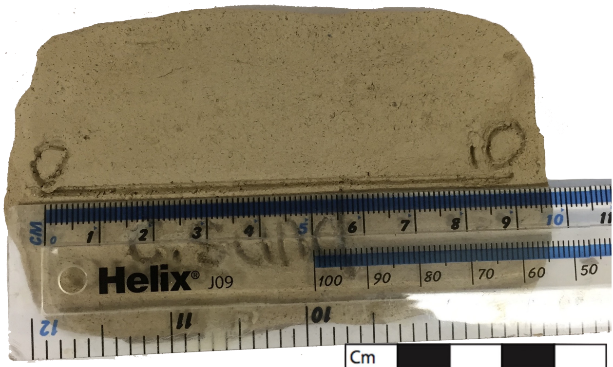
Figure 5.3 The clay slab showing the shrinkage of the line drawn in the wet clay from 10cm to 9cm after drying (Author's Photo).
