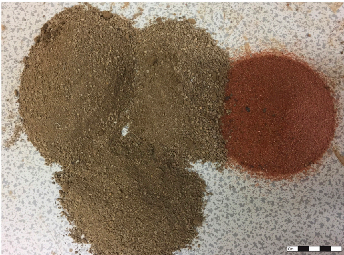
Figure 5.2 The sand and clay weighed out for the 30% temper vessel before being mixed with water and wedged (Author's Photo).
