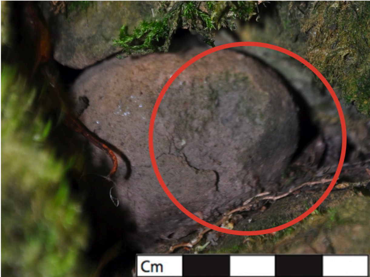
Figure 6.16 Vessel E15 with a frost fracture on the side after one month; the area of damage is within the red circle (Author's Photo).
