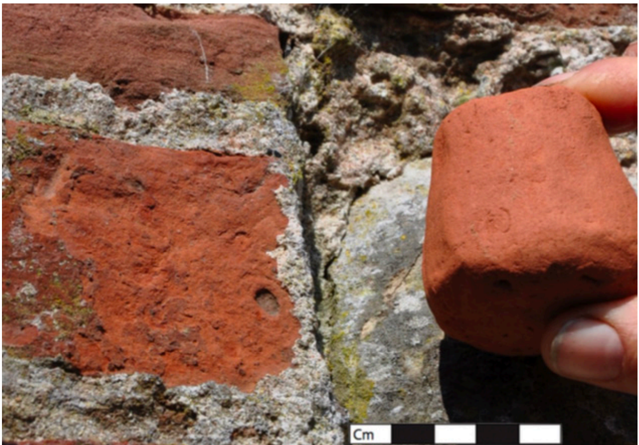
Figure 5.24 A test pot held next to an 18th century brick and the red local red sandstone above it showing the similarity in colour between the two fired clay objects and the local sand (Author's Photo).
