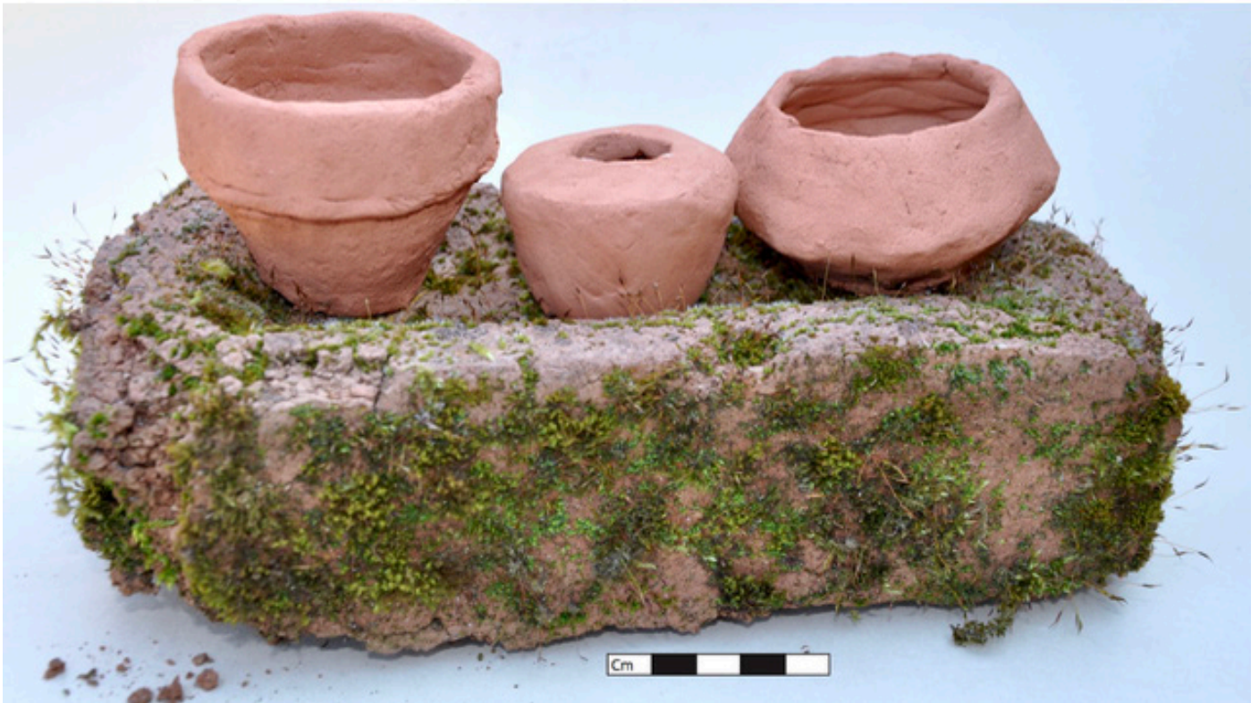
Figure 5.25 The fired clay vessel beside a poorly fired brick that has become weathered, showing the difference in colour between the paler, badly fired brick and the richer red coloured fired clay vessels (Author's Photo).
