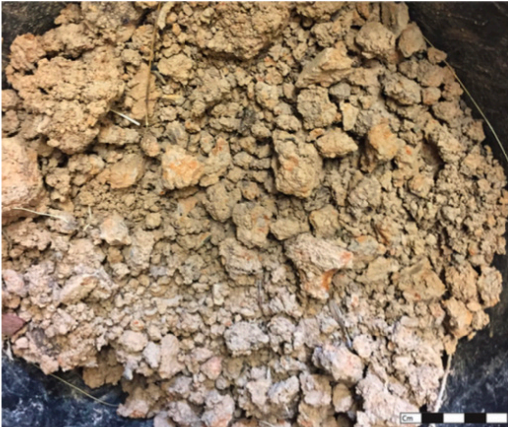
Figure 5.8 The clay, before being processed, is lumpy with traces of natural plant materials (Author's Photo).
