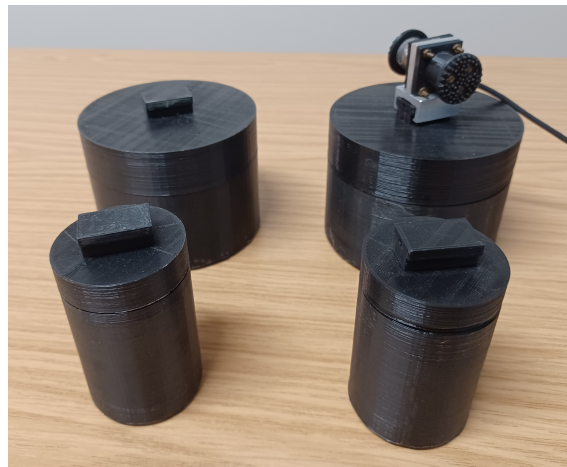
Figure 3.5: The objects used in the experiment. L-R 355g, 490g. Top right object has force transducer attached as it was prior to each lift.
