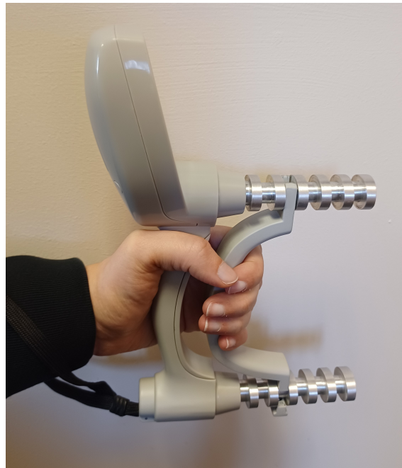
Figure 3.2: The Grip Force Dynamometer
