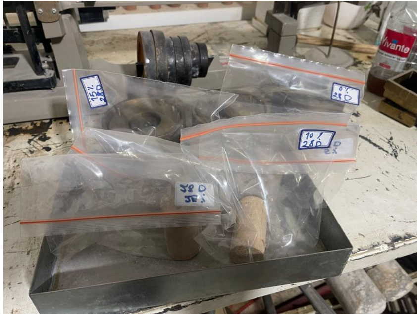
Figure 3- 5: Prepared samples for 28-day test
