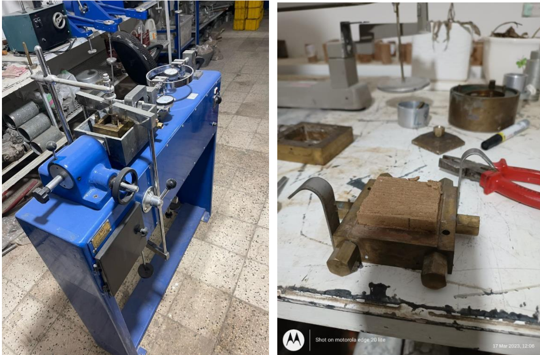
Figure 3- 4: Direct shear test device and it's sample
