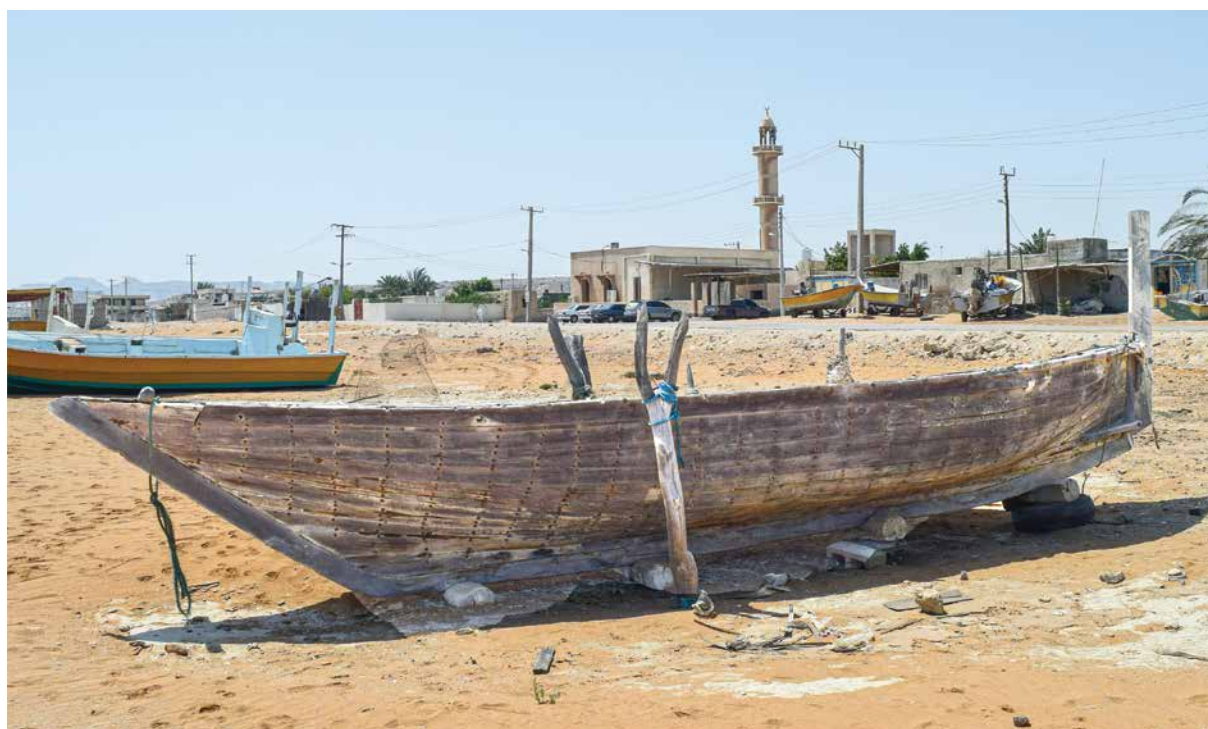
Fig. 6 The jalkash of Gambrun, island of Qeshm (length overall: 7.8 m; beam 2 m) (photo: S. Kalantar)
