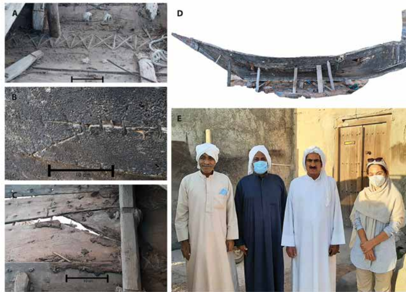
Fig. 2 The āmele of Bostane: (A) stitching of the keel; (B) the sewn and bitumen-coated hull planking; (C) planking and a frame from inboard, showing much damage to the stitching; (D) profile view – the length over all is 9 m and the beam 2.4 m; (E) Abdollah and Esmail Esmaili (first and second from left), sons and former assistants of the builder, together with Ebrahim Ahmadi (third from left), who introduced us to them, along with the lead author (right), in Bostane, 2021 (photo: M. Shorouj)
