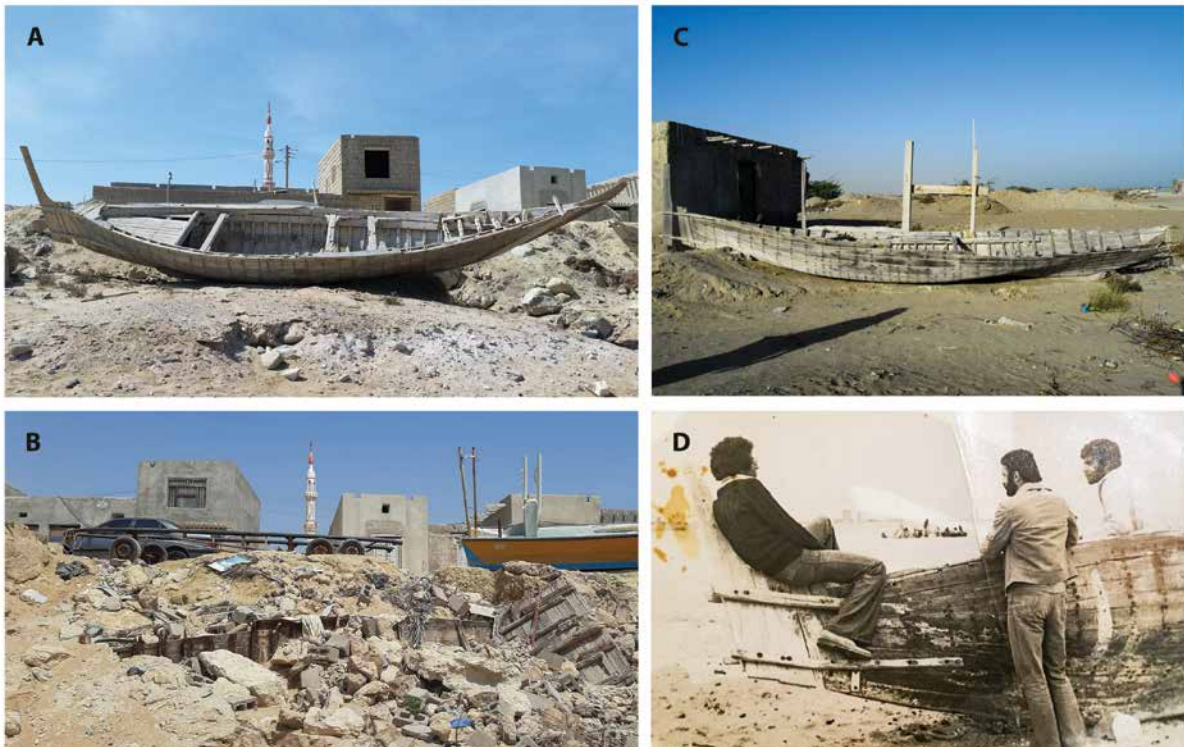
Fig. 5 The nailed baggāra : (A) an example at Ramchah in 2017; (B) the same vessel in 2022, having suffered significant damage; (C) one of two baggāras observed at Jask (preserved length 6.7 m; beam 1.2 m) (photos: S. Kalantar); (D) men at the stern of a baggāra in Jask in the 1970s (photo: courtesy of H. Heidari)
