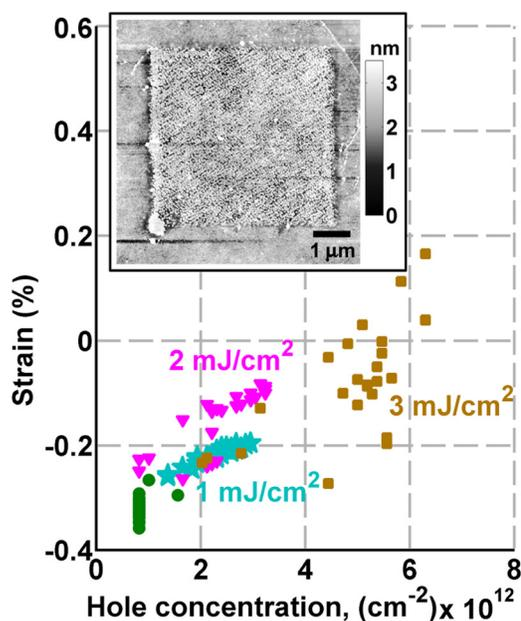
FIG. 3. Strain and carrier concentration induced by photoexcitation with  $1 \text{ mJ/cm}^2$  (cyan stars),  $2 \text{ mJ/cm}^2$  (magenta triangles), and  $3 \text{ mJ/cm}^2$  (brown squares) laser pulses extracted from correlated peak positions. Inset: AFM image of a sample after photomodification.
