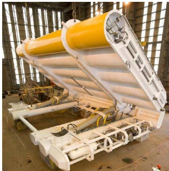
Figure 9 Oyster hydraulic pumps (Keysan, McDonald et al. 2010)
