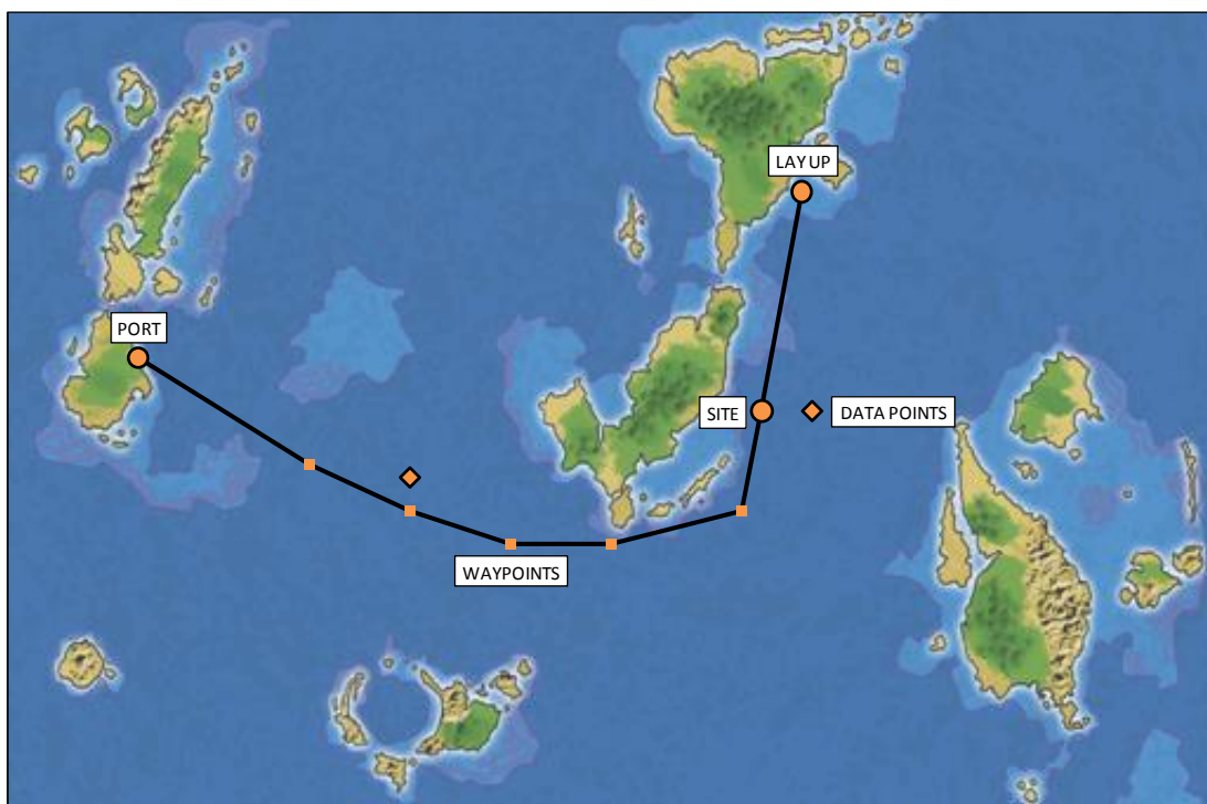
Figure 3-4: Spatial inputs including vessel transit way points and tracks, key locations and metocean data points (Map: Tipex, 2011)
