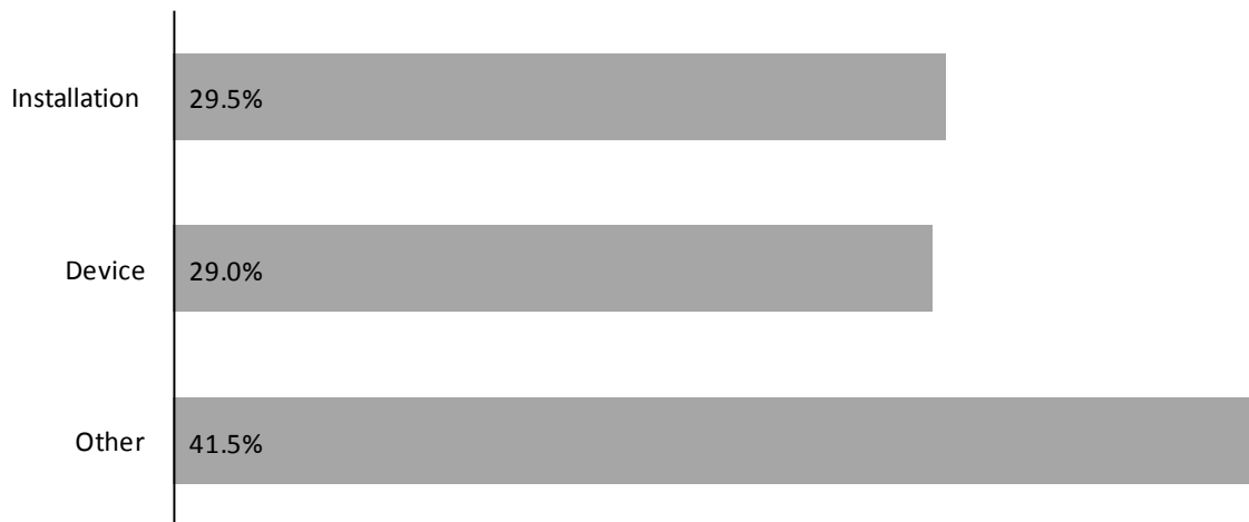
Figure 1-1: Installation and device costs as a proportion of the total project cost for a single wave energy converter
