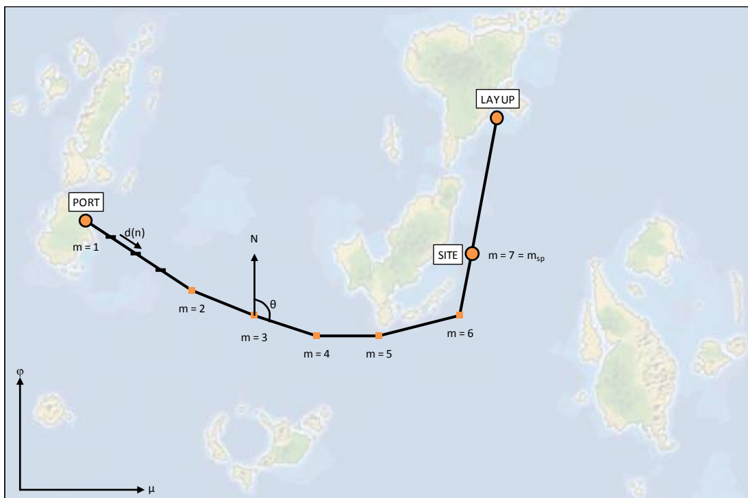
Figure 3-19: Transit parameters and their application, including d_{(n)} , the cumulative distance travelled and \theta the bearing of transit
