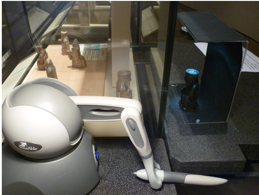
Figure 5.2: Two other strategies presented at ‘Touching the Untouchable’, allowing for physical (ghost touch, right) and virtual (haptic pen, front) explorations of a “Lewis Chessmen” piece.
