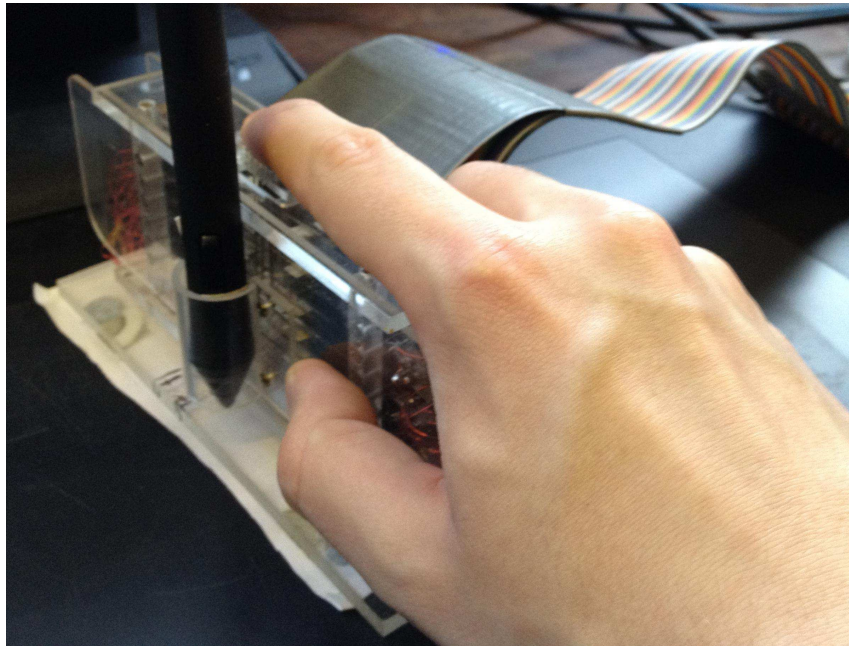
Figure 6.2: How the tactile display is held during use.
