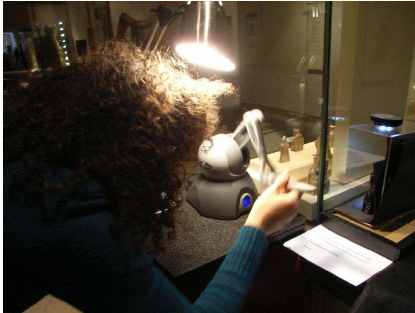
Figure 5.7: Use of the haptic pen setup to explore the surface of the “Lewis Chessmen” piece.
