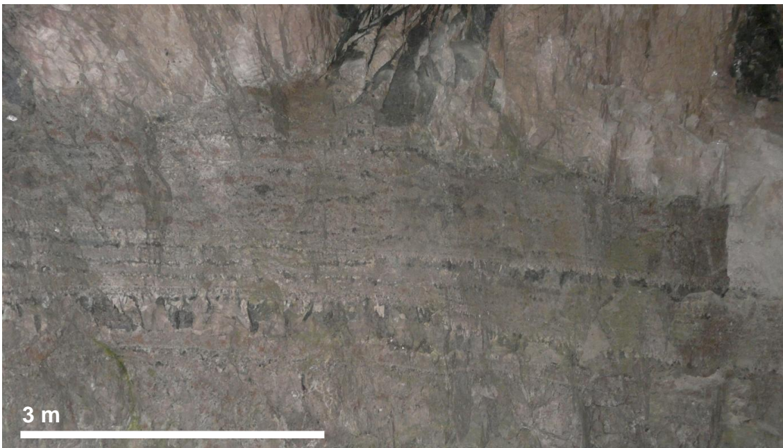
Fig. 2.3.3 Zoning; Massive K-feldspar outer core (top), with intermediate zone of quartz/plagioclase with garnet crystallisation horizons (line rock). Crystallisation propagation appears to be downwards. Li Gruva pegmatite
