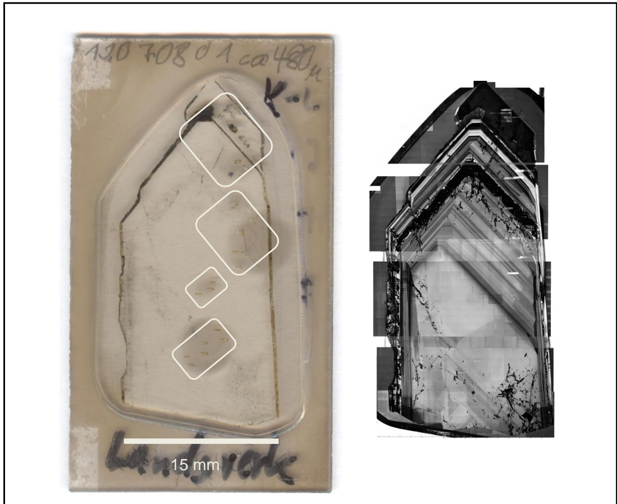
Fig. 4.6.8 Scan of a thick section of a hydrothermal quartz crystal from Landsverk 1, with corresponding CL-SEM image. The rounded rectangles indicate regions containing LA-ICP-MS ablation sites
