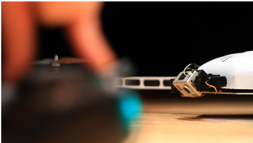
Figure 15: Remote control over the tilt function of Skybot 's onboard camera – full radio linkup to a mini monitor on the gyro-controller gives the camera operator on the ground an image direct from the camera in the air.
